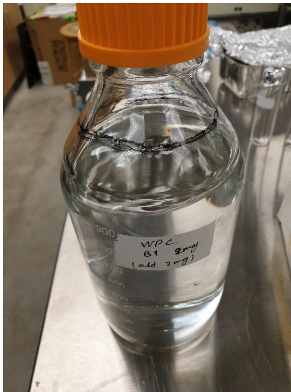
Figure B.9 Carbon buildup at bottle rim with dry powder dosing
