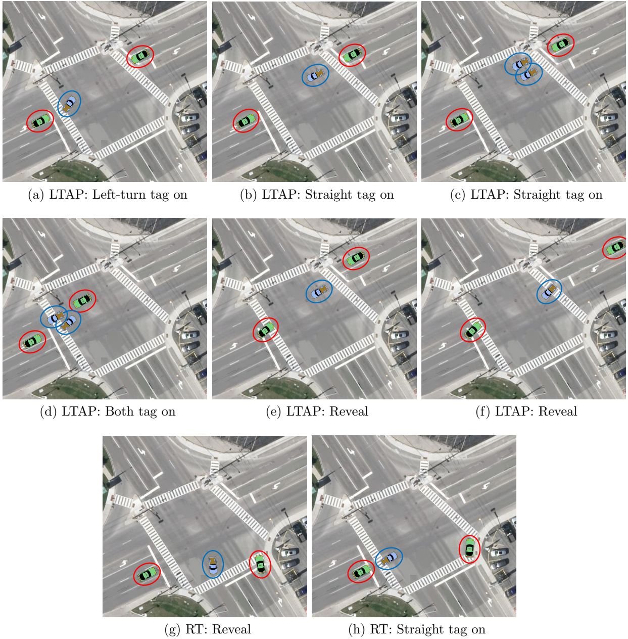
Figure 5.4: Example configurations for each of the occlusion situation categories laid out in the taxonomy in figure 5.3. The blue circles represent the SOVs, while the red circles represent the vehicles occluded from each other by the SOV.
