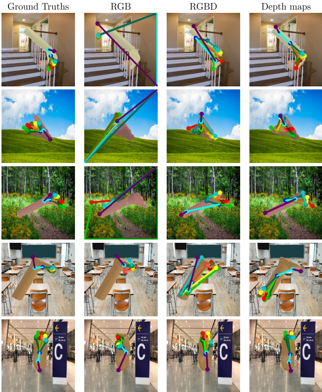
Figure 4.3: Examples of joint detection generated by our system. First column shows the expected joints' positions, while the other three show the output for different types of input. Each row shows a different example.
