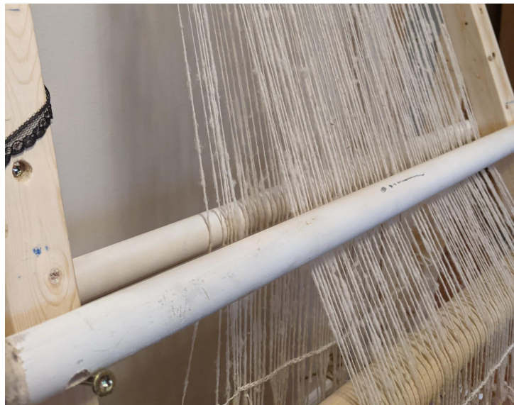
Fig. 78: Temporary spare rod placed behind the back warp and anchored to the loom. Credit: Tatianna Bechal, 2021.
