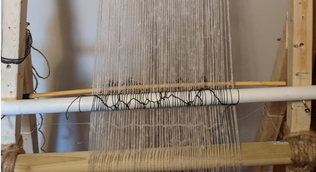
Fig. 84: The first lease setup after several threads have broken. The lease has become uneven over time due to several broken warp threads. Credit: Tatianna Bechal, 2021.
