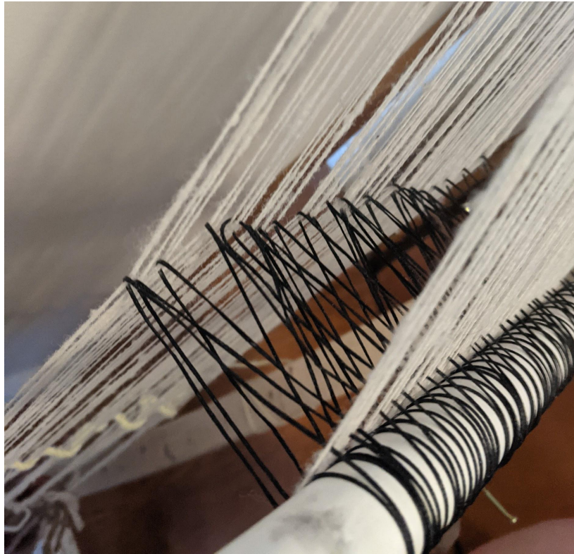
Fig. 80: The heddle and leash are set up and the temporary spacer bar has been removed. The odd threads can be pulled forward between the even threads when the weaver pulls the heddle bar towards themselves. Credit: Tatianna Bechal, 2021.
