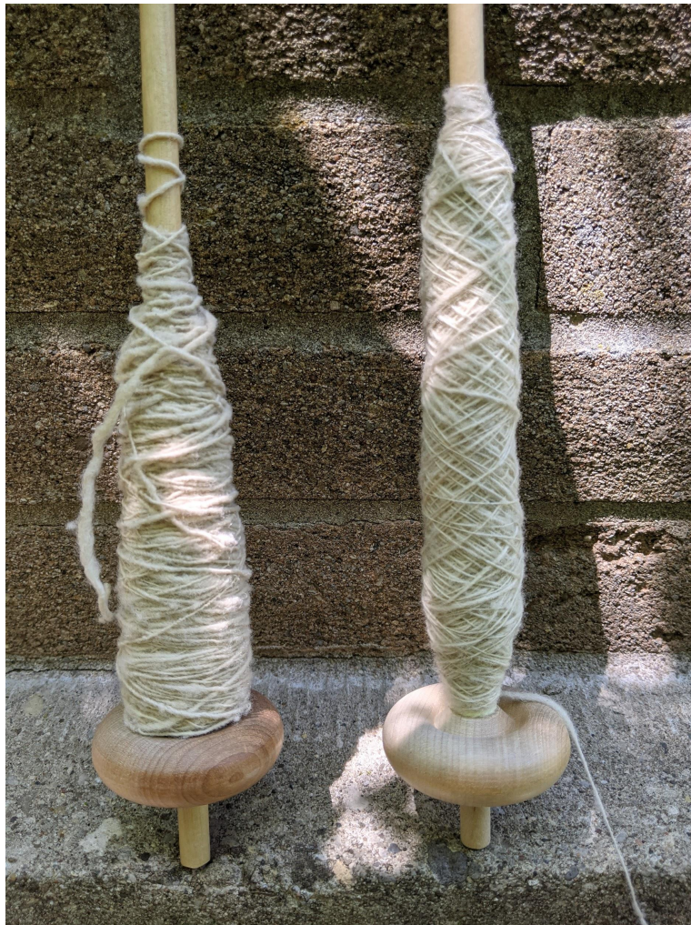
Fig. 60: The very first spindle (left) contrasted to the fourth spindle (right). The threads on the left spindle are bulky and uneven, while the thread on the right spindle is much finer, more consistent, and more tightly spun. Credit: Tatianna Bechal, 2021.
