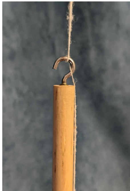
Fig. 57: Small hook at the top of the spindle keeps the thread securely attached to the spindle as it spins. Credit: Tatianna Bechal, 2021.
