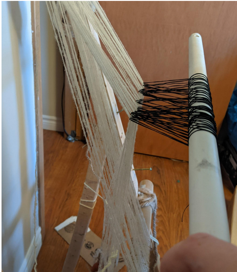
Fig. 81: The heddle is completely set up with a functioning counter shed. Credit: Tatianna Bechal, 2021.
