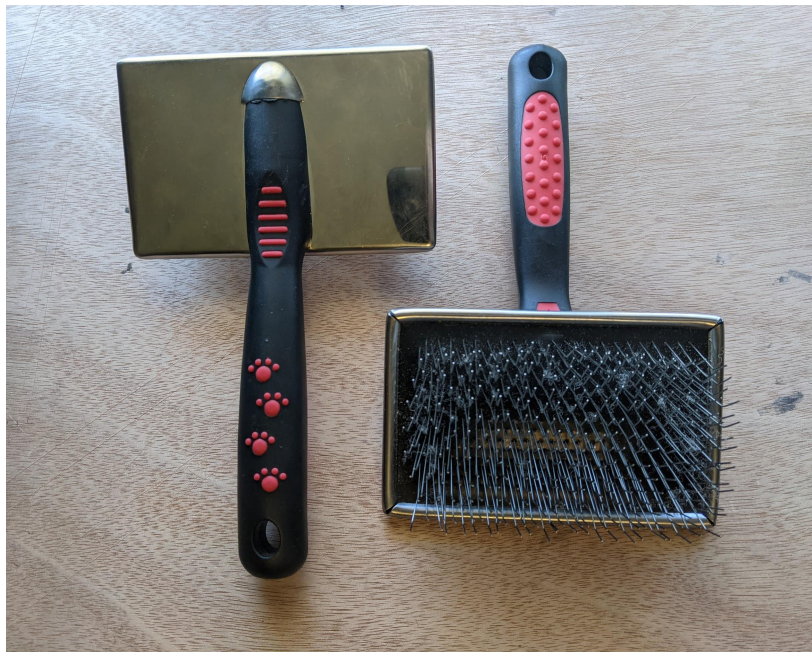
Fig. 35: Pet grooming brushes. The teeth are very similar to the teeth found on carding brushes. Credit: Tatianna Bechal, 2021.
