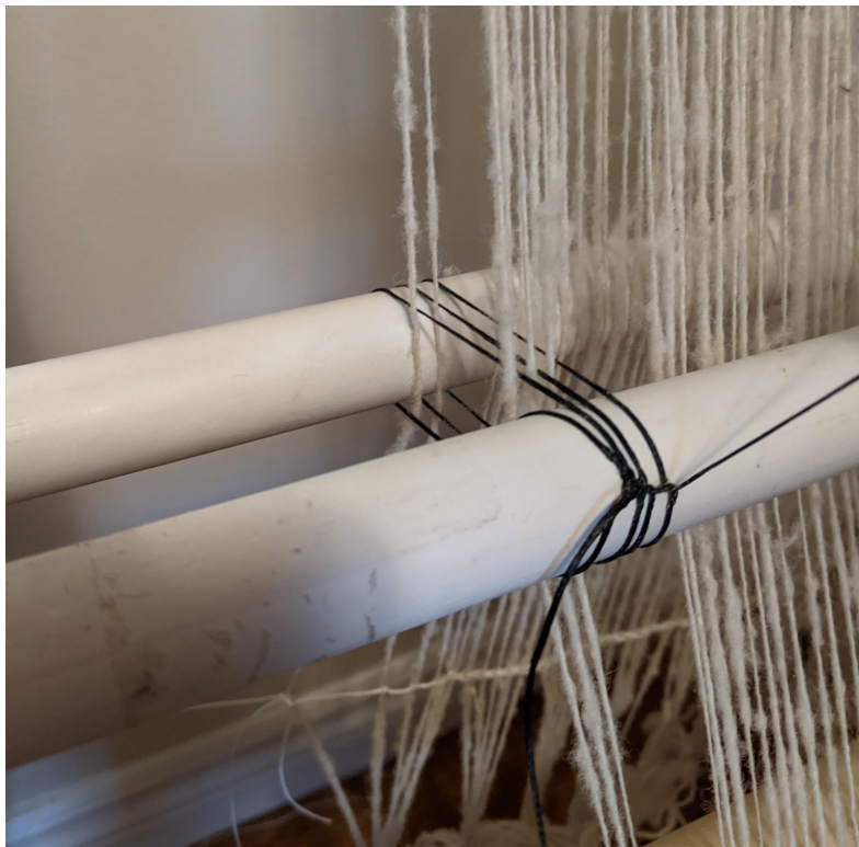
Fig. 79: The leash (black thread) is being tied to the heddle bar in front, passing between alternating odd and even warp threads. Behind the odd warp threads in the back rests a temporary rod used to space out the leash and control the tension. Credit: Tatianna Bechal, 2021.
