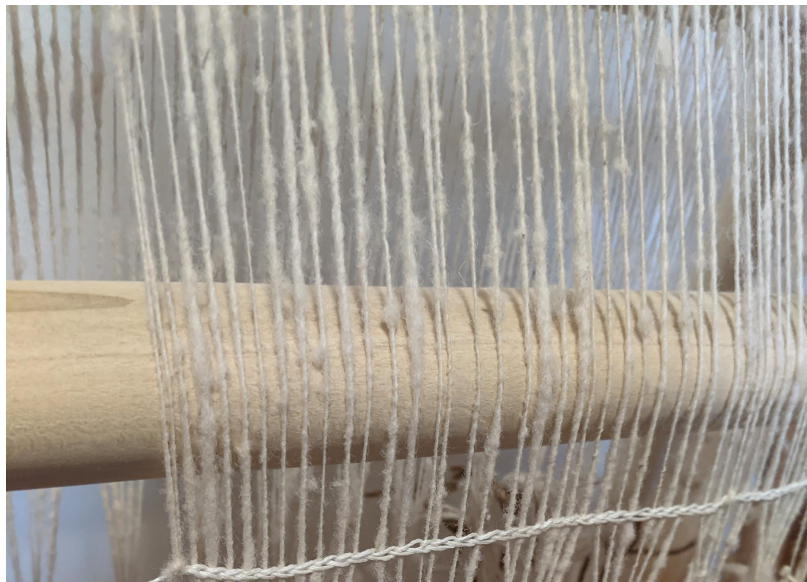
Fig. 70: The warp beam holds one set of threads (even threads) forward and away from the other set (odd threads). Credit: Tatianna Bechal, 2021.
