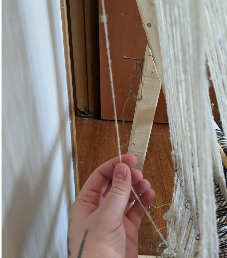
Fig. 75: Even after taking multiple days setting up the heddle an entire odd warp thread was missed in the leash. Credit: Tatianna Bechal, 2021.
