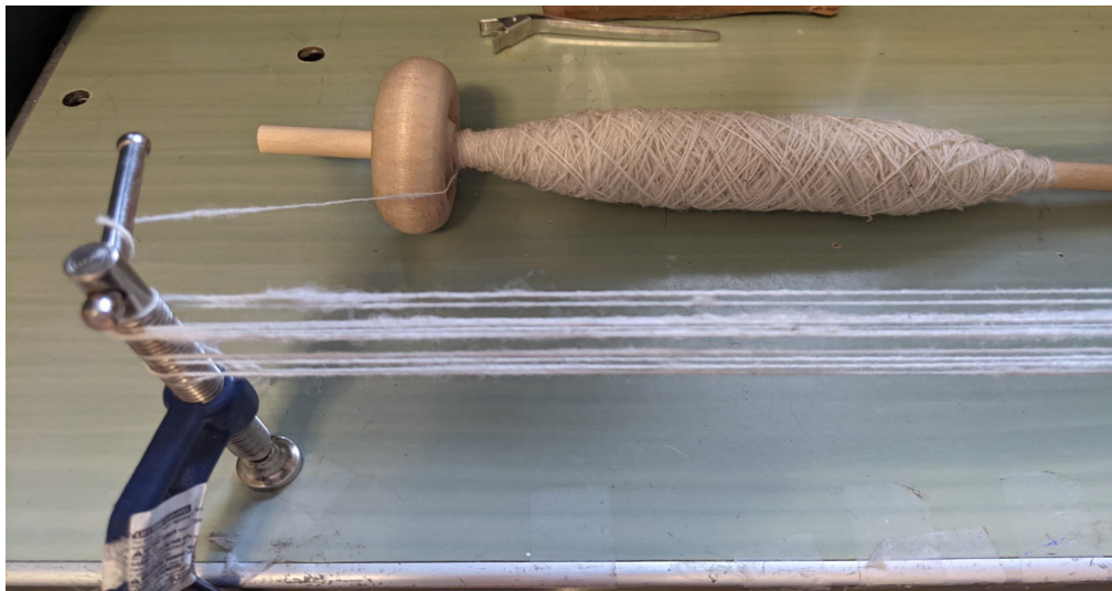
Fig. 66: The second attempt at measuring out warp threads using a more controlled method, measuring out only a few threads at a time. Credit: Tatianna Bechal, 2021.
