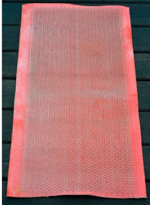
Fig. 32: Carding cloth teeth closeup from Okanagan Dye Works. © 2021, Okanagan Dye Works.
