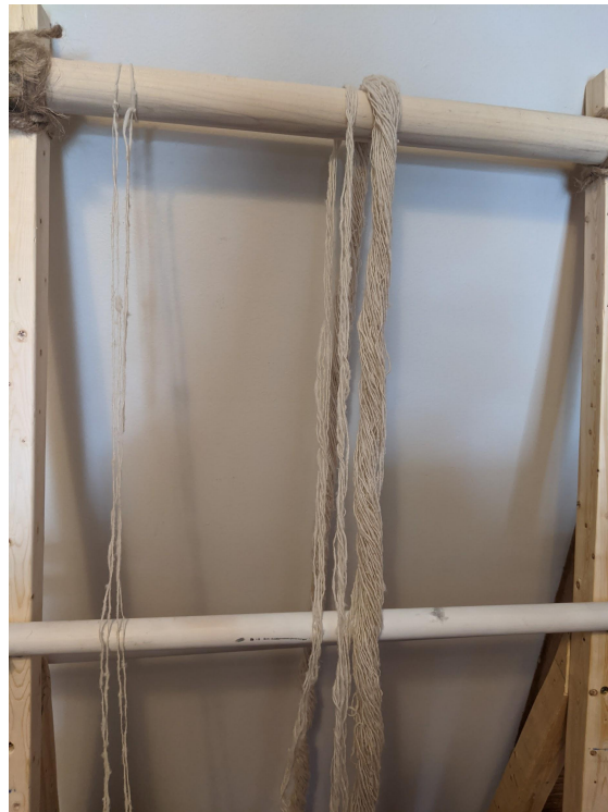
Fig. 67: The undressed loom showing the first few warp threads attached. The warp threads are measured and cut to length. Credit: Tatianna Bechal, 2021.
