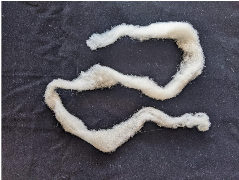
Fig. 47: A small roving made using brushes and epinetron . Credit: Tatianna Bechal, 2021.
