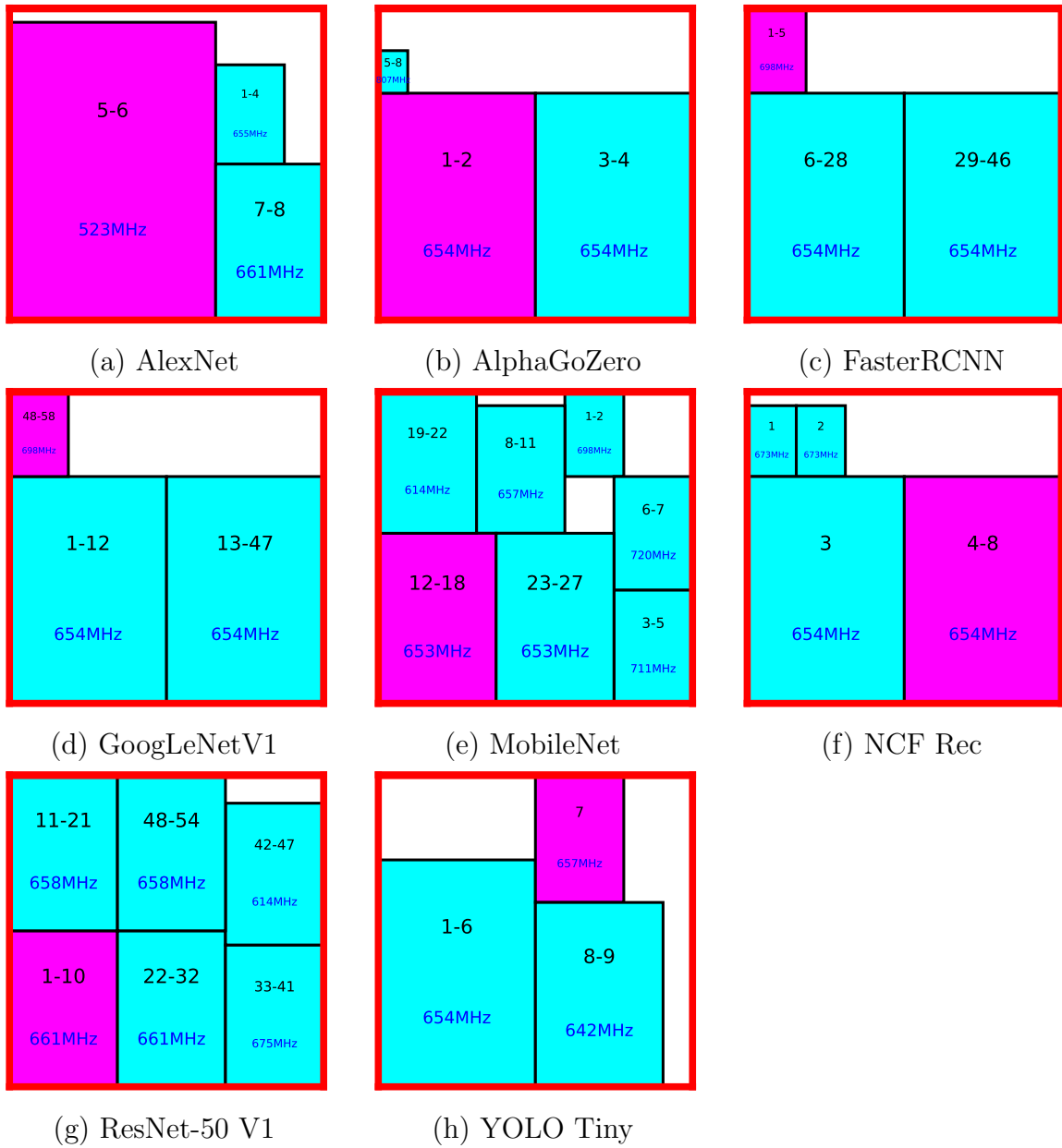
Figure 5.5: Partitioned solutions of every topology with the xcvu37p-6-times-y profile on VU37P
