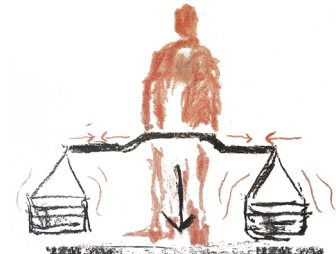
the typical barbell forces the user to conform to its standard during a lift. The proposed design allows the length of the weight to be modified accordingly to the user's height
