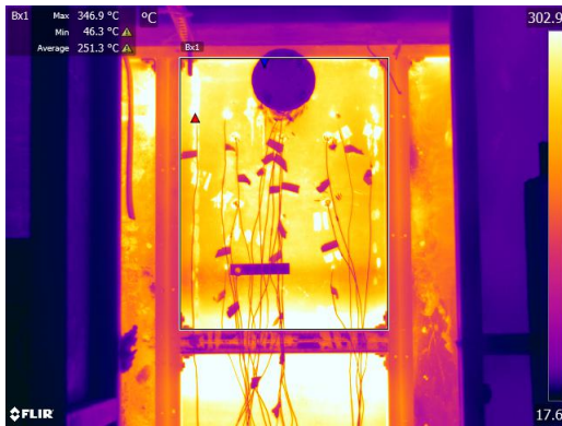
(a) IR image of the unexposed side at 14 minutes of test 6 with no insulation. Average temperature 251 °C
