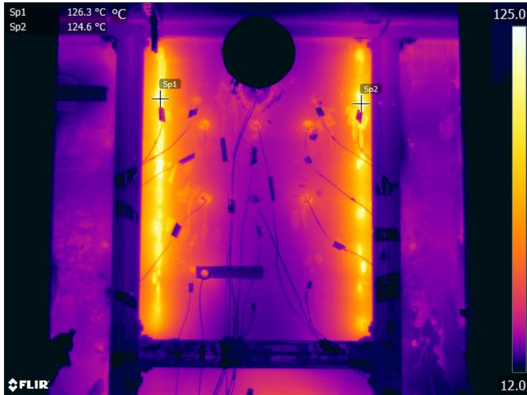
Figure 4.46: Test 10: IR image at 15 minutes, \epsilon= 0.85 , 5 IMO wall stiffener monitoring points
