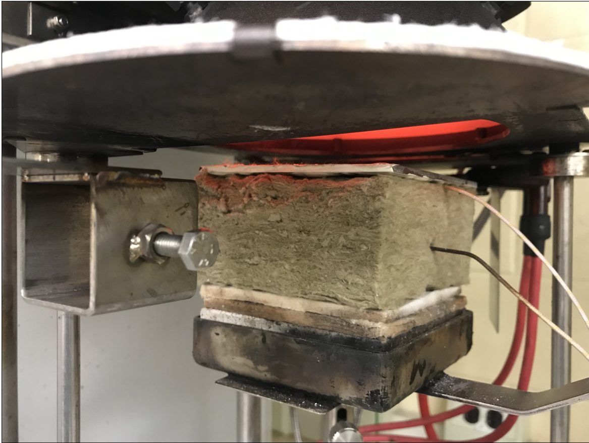
Figure 3.27: Insulated cone test- scenario 1 test setup
