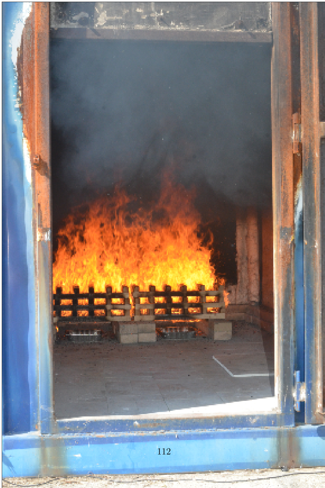
Figure 4.9: Photo showing representative flame height of the two SBS crib configuration
