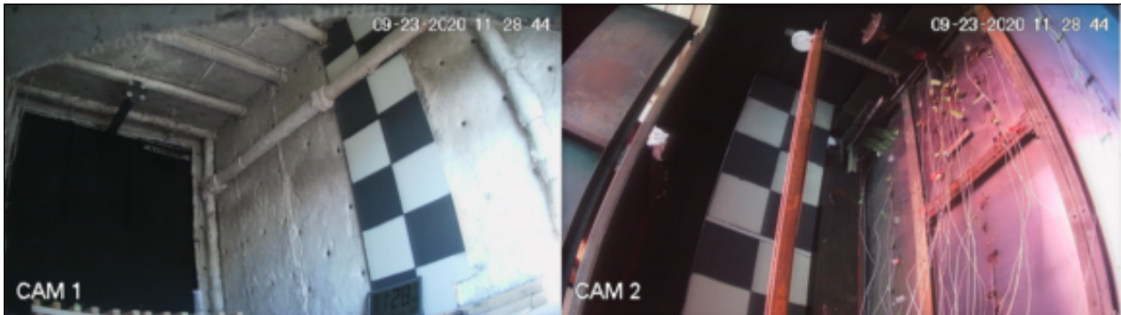
Figure 4.7: Video capture of Test 3, with smoke detector shown mounted in the transition compartment
