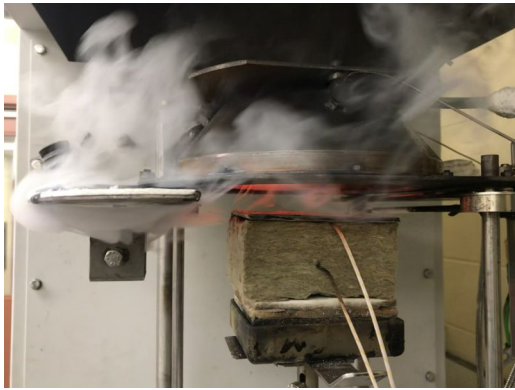
(a) Cone calorimeter scenario 1: Smoke production prior to ignition
