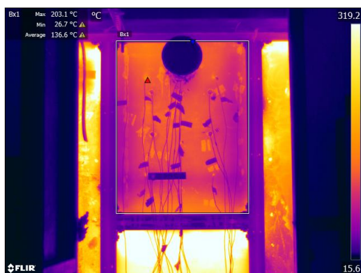
(a) IR image of the unexposed side at 7 minutes of test 6 with no insulation. Average temperature 136 °C
