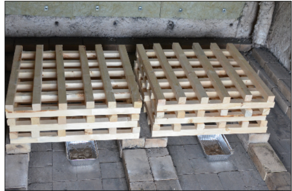
(b) Fuel tray configuration - two side by side wood cribs
