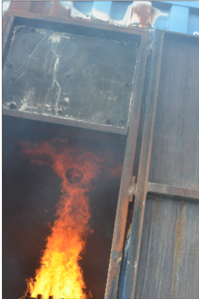
Figure 4.3: Photo of flame impingement on the ceiling with the two stacked crib configuration during Test 2
