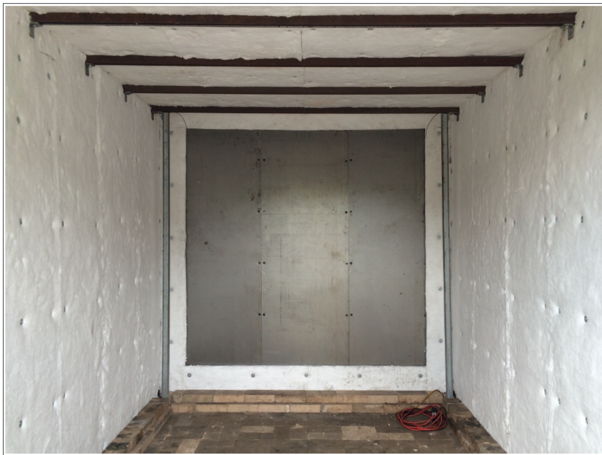
Figure 3.4: Panels shown installed in the wall test apparatus [8]
