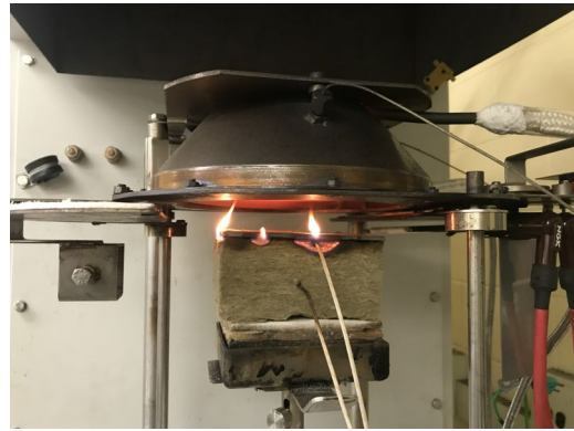
(b) Cone calorimeter scenario 1: sustained burning following ignition
