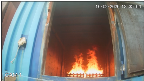
(a) Test 7: Video still at t=15 min looking into the fire compartment
