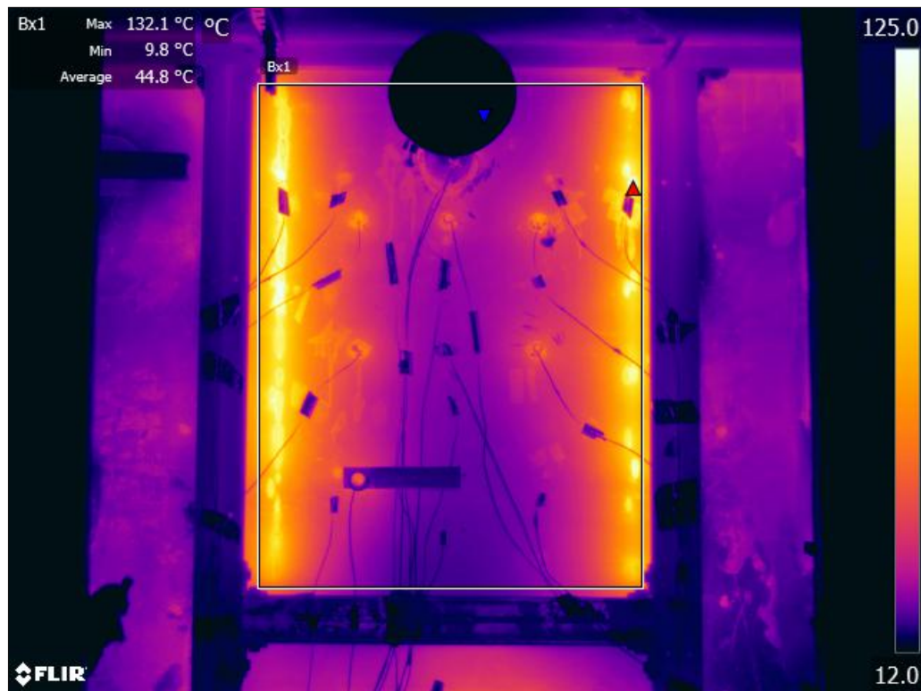
Figure 4.42: IR image at 15 minutes of Test 10 with IMO A-15 insulation fitted, showing an average surface temp of 45 °C in the test area of interest
