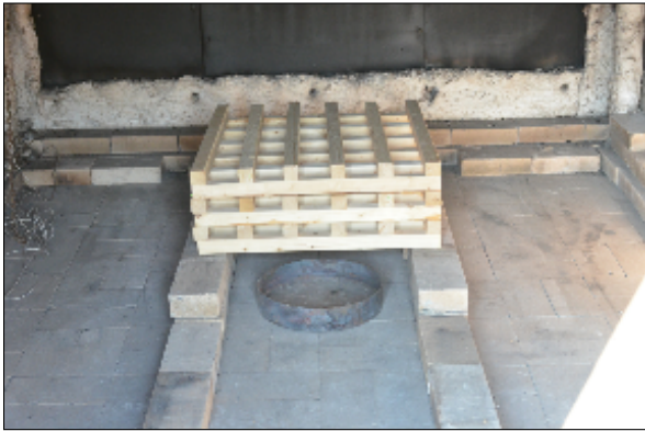
(a) Fuel tray configuration - single and two stacked wood crib configuration
