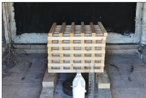
(b) Two stacked cribs stacked configuration in the wall test unit
