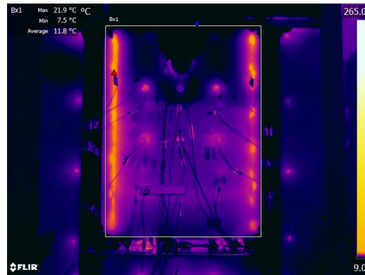
(b) IR image of the unexposed side at 6 minutes of test 10 with IMO A-15 insulation, scale matched to uninsulated test image. Average temperature 12 °C
