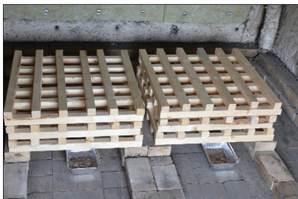
(a) Two wooden cribs in a side by side (SBS) configuration in the wall test unit
