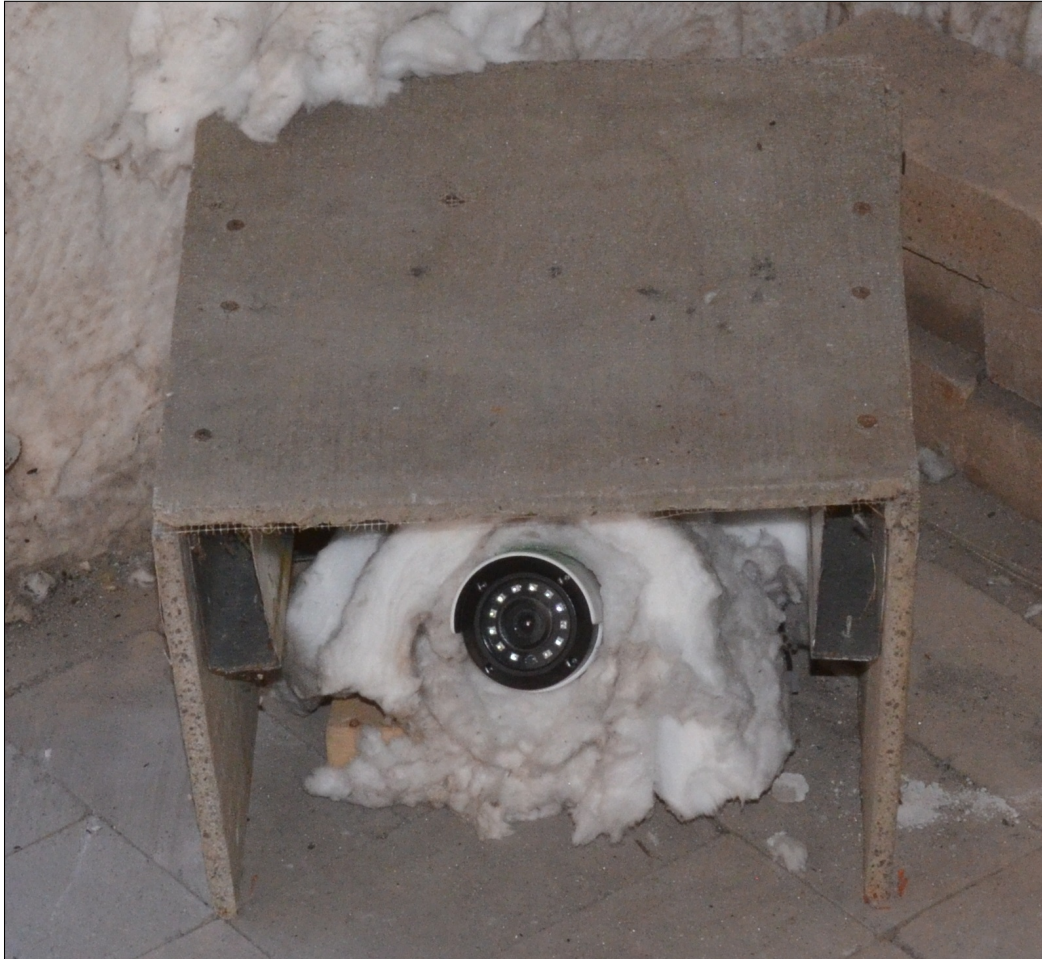
Figure 4.5: Photo showing additional camera protection used for tests 3 and 4
