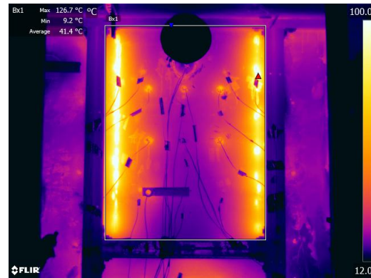
(b) IR image of the unexposed side at 14 minutes of test 10 with IMO A-15 insulation. Average temperature 41 °C
