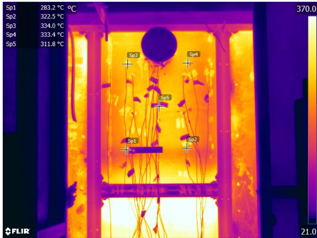
Figure 4.44: Test 6: IR image at 12 minutes, \epsilon = 0.85 , 5 IMO monitoring points shown (Note center quadrant point obscured)
