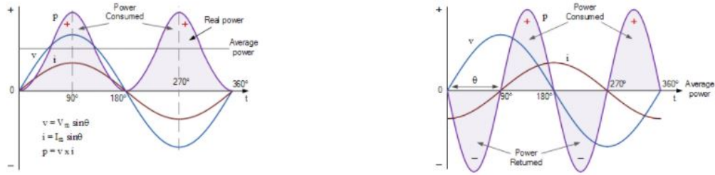
(a) Power loss from a resistive element
