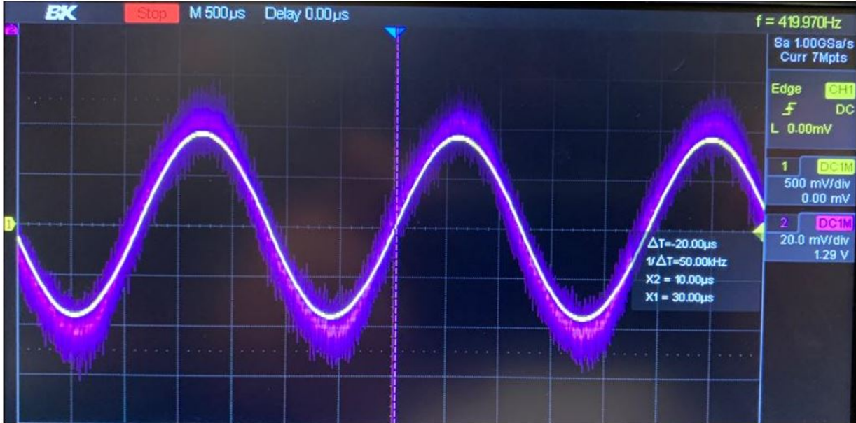
Figure 5.7: At 420Hz, the voltage and current waveforms overlap each other with a 20μs (or 3.024°) shift
