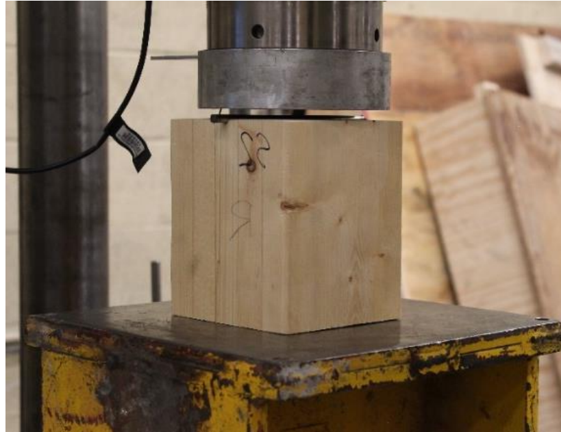
a) Embedment Test Setup
