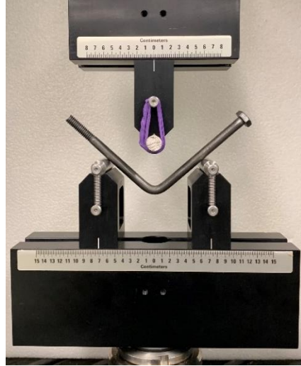
a) Three-Point Bending Test Setup
