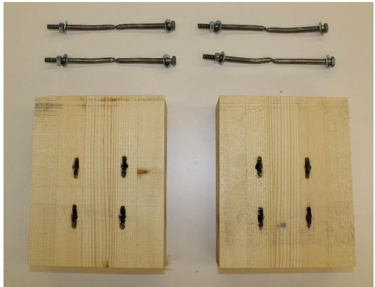
b.) Embedment and Damaged Bolts
