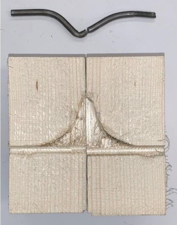
a.) Wood Crushing and Bent Bar
