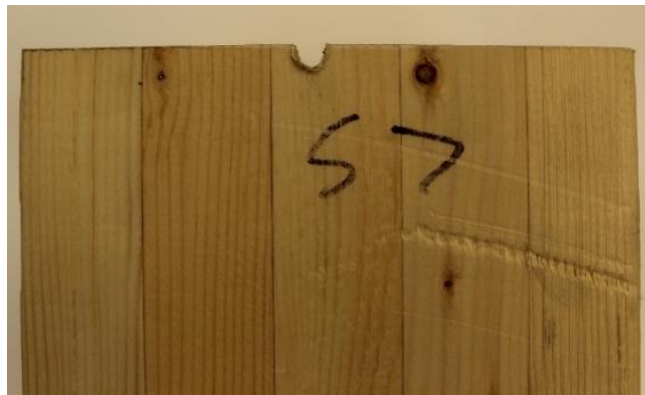
b) Embedment Failure
