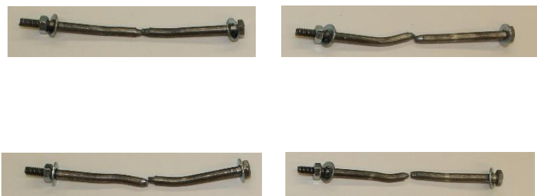
c.) Deformed Bolts Broken at Center Hinge
