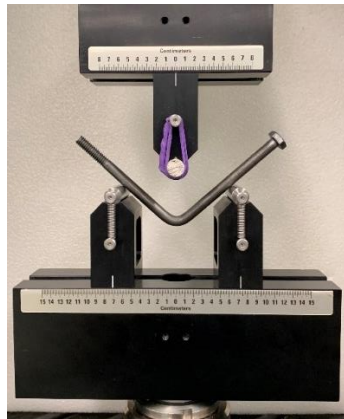
c) Damage After Unloading - Steel
