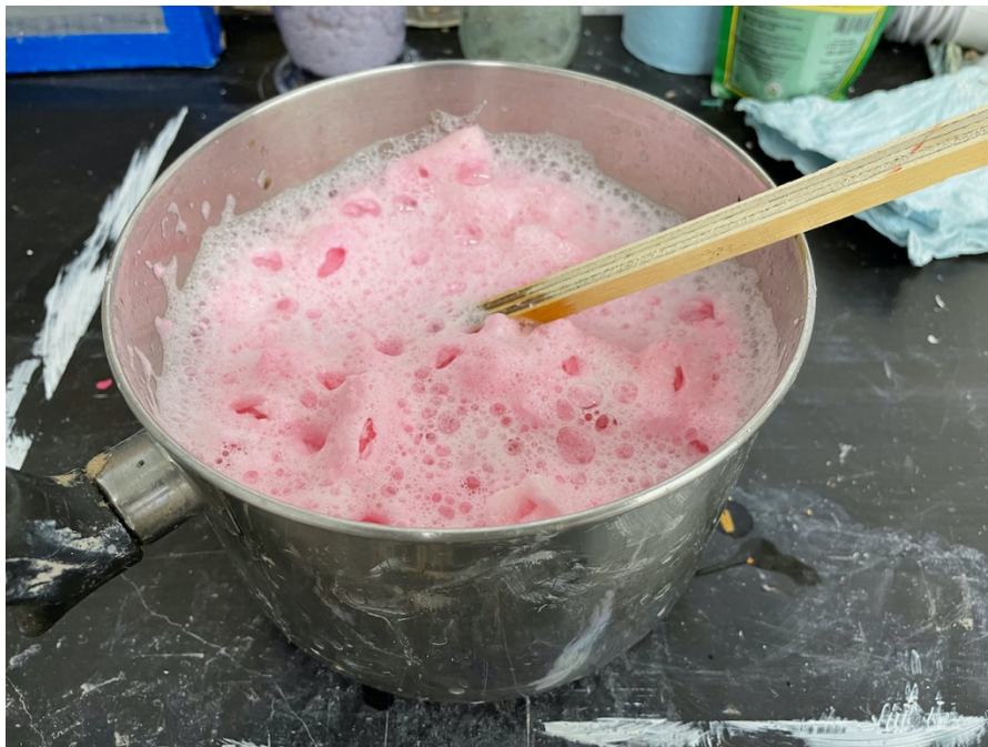
Fig. 17. Compostable pink packing peanuts are shown dissolved in water. They were later added to white paper pulp, creating a pale pink tint.
