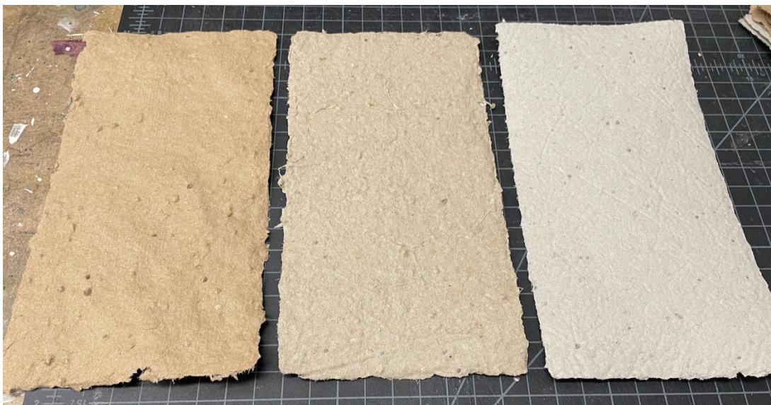
Fig. 18. Different colours of handmade paper. On the left, paper made from cardboard boxes; on the right, paper made from egg cartons; and in the middle, paper made from a mixture of both.
