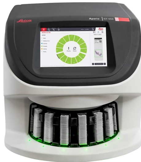
Figure 2.1: A digital pathology scanner. WSI scanners are capable of producing high quality images of multiple slides at the same time. Image taken from Leica Biosystems official website
