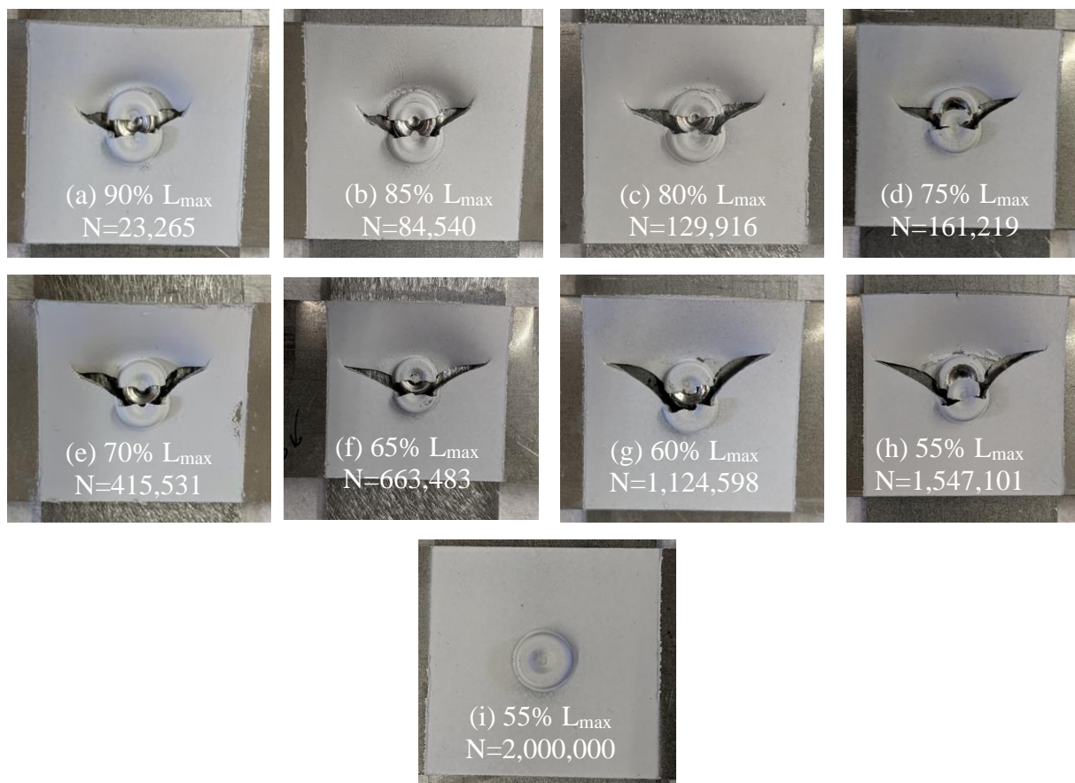
Figure 38: Al 6016 2mm by 1mm SPR cross-tension post fatigue test 45° clenched sheet details of varying load levels undamaged runout (i)
