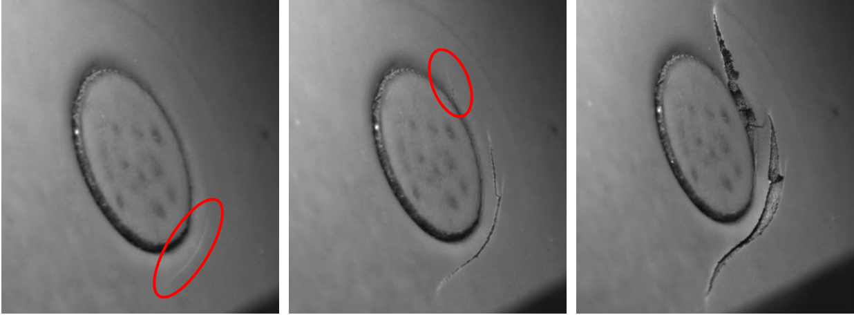
Figure 59: Pierced sheet details from N_{final} = 263,122 45^\circ specimen in Figure 57 with first visible crack at N = 188,000 (a), propagated first crack and visible second crack at N = 240,000 (b), and frame before separation (c)
