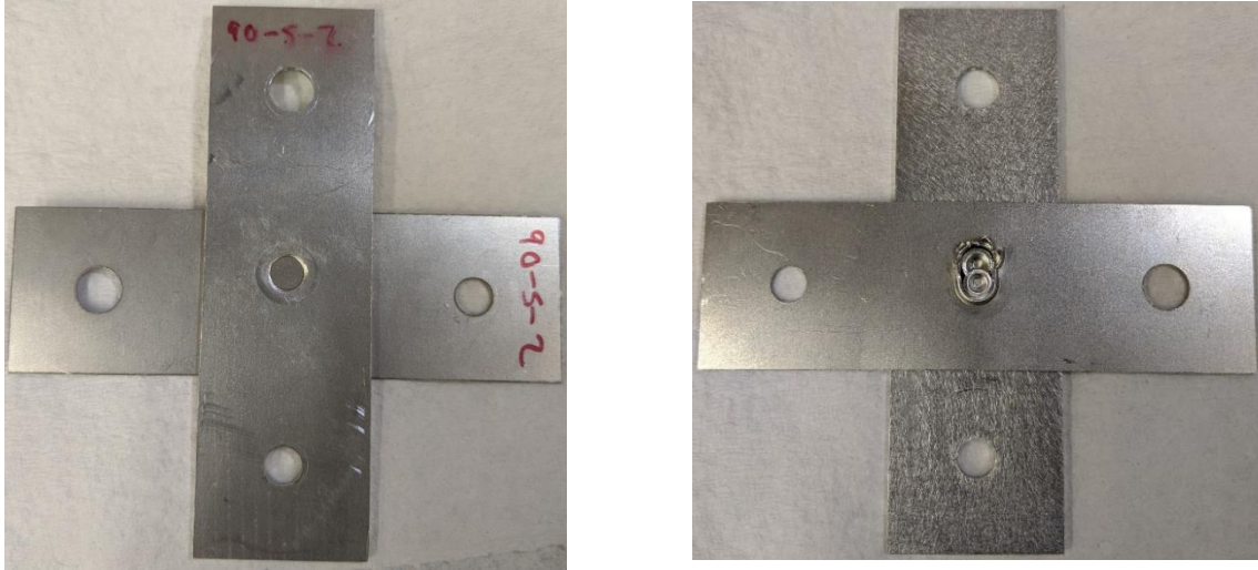
Figure 23: Al 6016 2mm by 1mm SPR cross-tension post quasistatic test 90° test pierced 2mm sheet (left) and clenched 1mm sheet (right)
