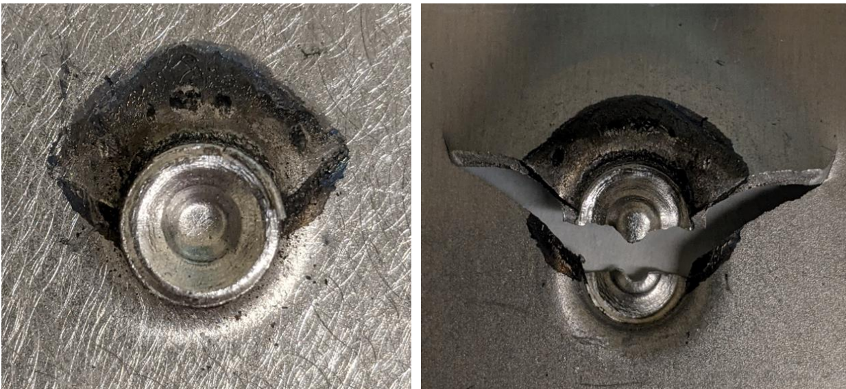
Figure 44: Fully separated Al 6016 2mm by 1mm SPR cross-tension 90^\circ specimen N_{\text{final}} = 415,531 2mm pierced sheet (left) and 1mm clenched sheet (right) fretting damage at sheet contact interface
