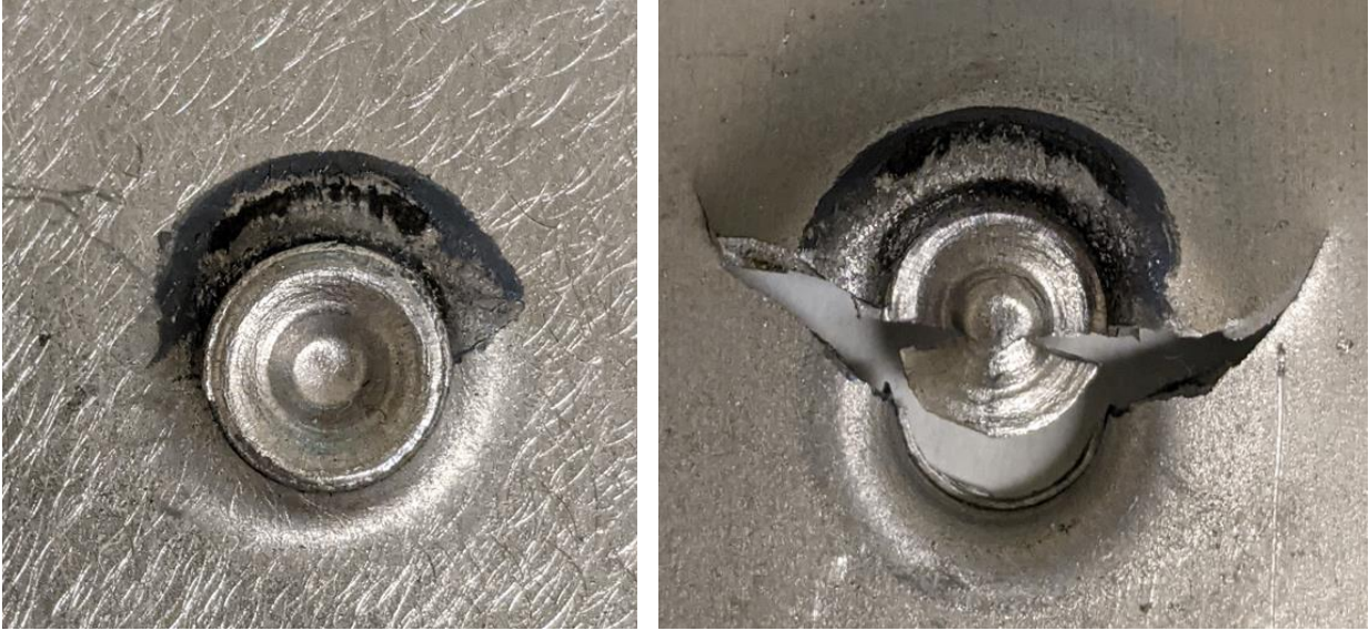
Figure 45: Fully separated Al 6016 2mm by 1mm SPR cross-tension 45° specimen N_{final} = 83,947 2mm pierced sheet (left) and 1mm clenched sheet (right) fretting damage at sheet contact interface
