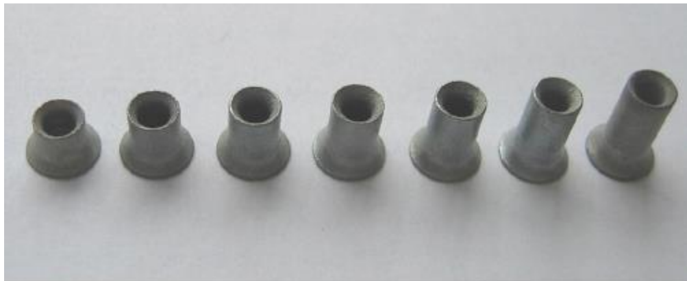
Figure 1: Typical pre-process SPR with varying length. Note sharp edge at open end for sheet piercing and countersunk closed end [2]
