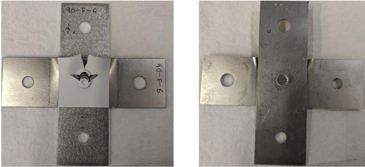
Figure 34: Al 6016 2mm by 1mm SPR cross-tension post fatigue test 90° test pierced 2mm sheet (left) and clenched 1mm sheet (right) N_{final} = 110,571
