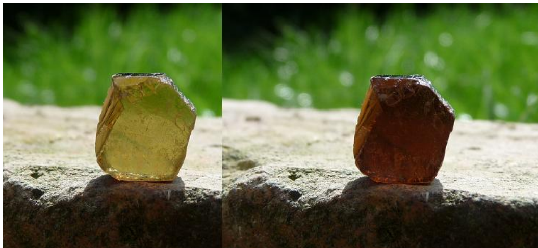
Figure 3.6: An example of optical dichroism in tourmaline. Photos are taken from the same spot and angle with the same illumination, but with the different orientation of the camera's polarizing filter. For one polarization, light absorption by the tourmaline crystal is stronger than for a perpendicular polarization, and the crystal appears darker. Reprinted from Wikimedia.
