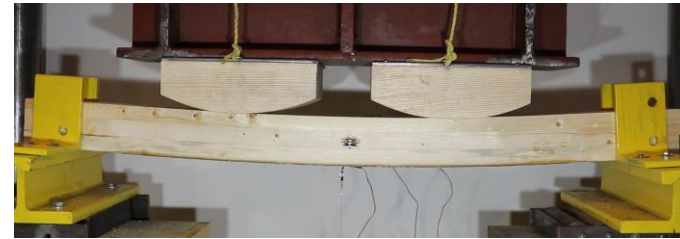
(4) Ultimate failure – horizontal shear in shear region
