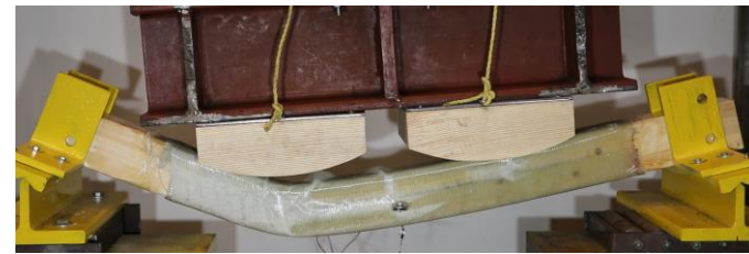
(4) FRP and wood failure propagation at third load peak
