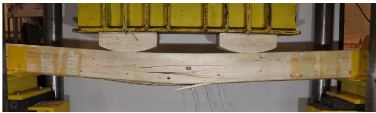
(3) Wood tensile failure *String pot disconnects
