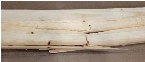
(c) Close-up of damage for U-01
