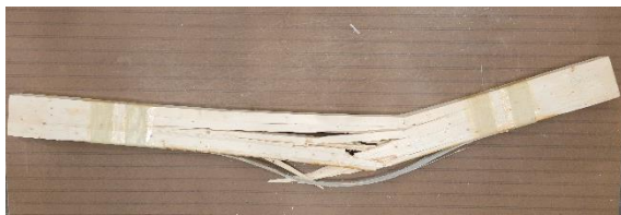
(b) Ultimate failure of R11-01
