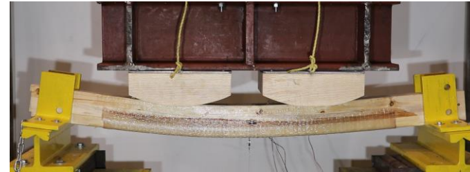
(4) Shear failure propagating along the beam
