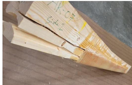
(b) Close-up of damage for R4-01
