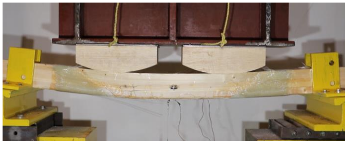
(3) Wood tensile failure under the point load
