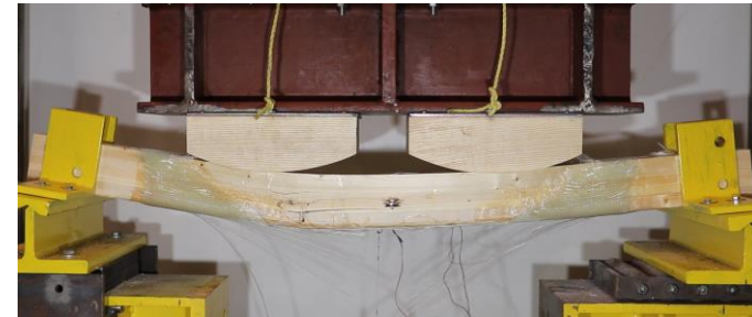
(4) Propagating wood failure and initiating of FRP rupture
