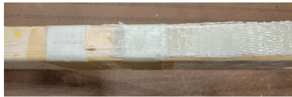
(c) Slipping of FRP on the tension face of R11-02
