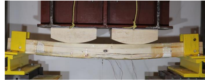
(4) Wood failure propagating through laminates
