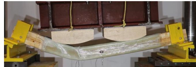
(4) FRP failure propagation and wood (tension and compression) failure confined near the leftmost point load
