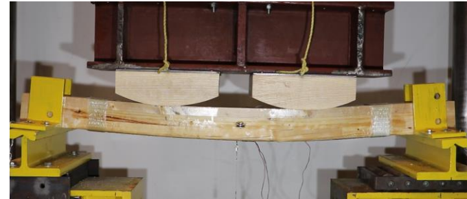
(4) Shear failure propagating throughout laminates
