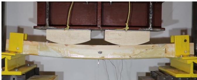
(3) Failure in the shear region
