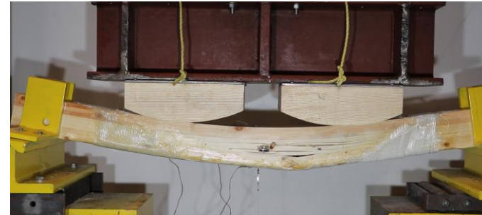
(4) Failure propagating into the shear region
