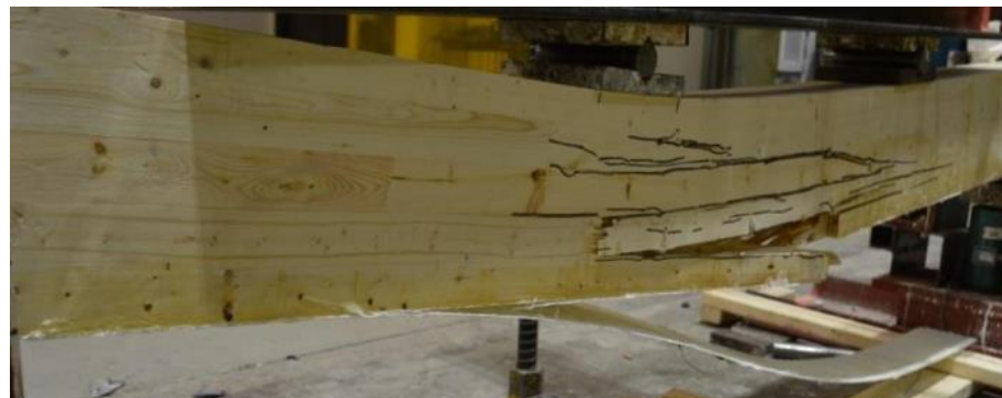
(c) Representative example of premature de-bonding of FRP due to the wood (Lacroix, 2017)
