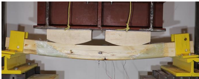
(3) Wood tensile and shear failure
