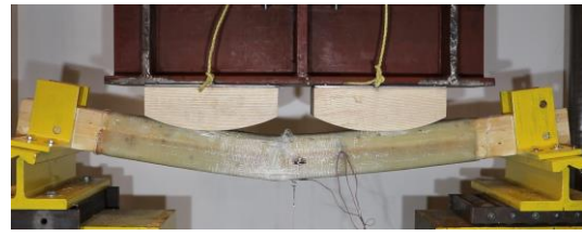
(b) Tension failure for R7-02
