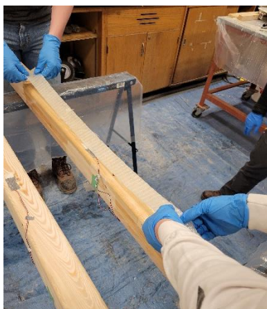
(c) Application of the FRP
