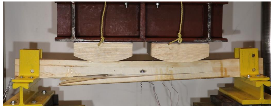
(b) R1-01 at initial failure
