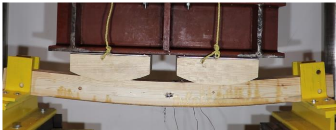
(3) Horizontal shear failure
