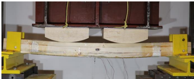
(3) Wood tensile and shear failure extending to shear hoop
