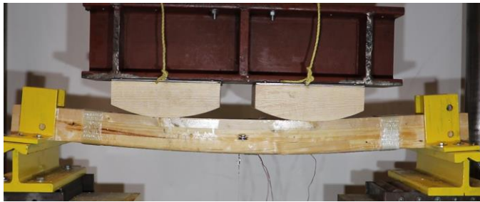
(3) Failure initiating in the tension laminate and extending to the shear hoop
