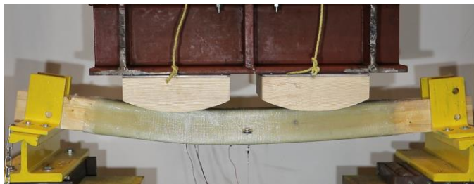
(3) FRP compression failure propagation within confined region
