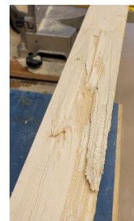
(c) Damaged laminates
