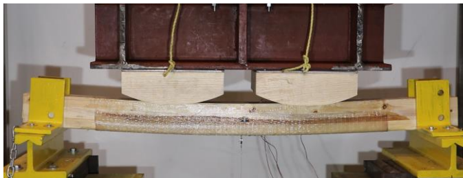
(3) Horizontal shear failure
