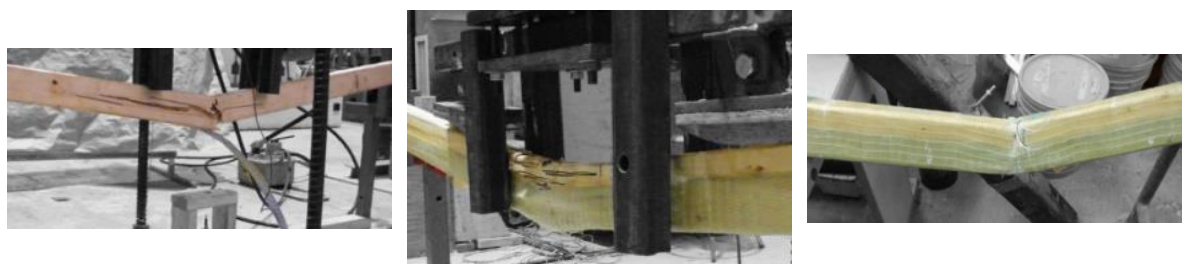
(a) Simple tension: FRP delamination
