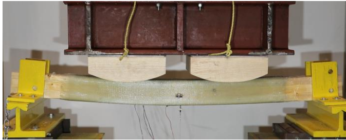
(2) Initial buckling of the FRP in compression near point load at maximum load ( P_{max} )
