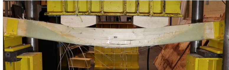
(4) Propagating wood failure and commencement of FRP tensile rupture
