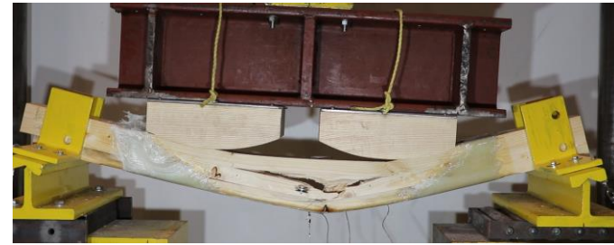
(4) Propagating wood failure and engagement of FRP shear reinforcement
