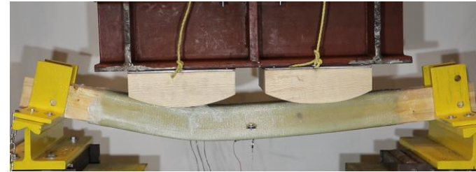
(4) FRP failure propagation and wood (tension and compression) failure confined near the leftmost point load
