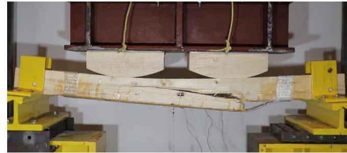
(3) Ultimate failure – large knot on tension face of the wood
