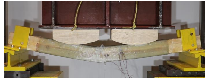
(4) FRP failure propagation and wood (tension and compression) failure confined at midspan
