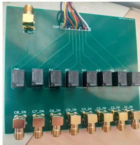
Figure 13: Relay switch for sensor bias and output
