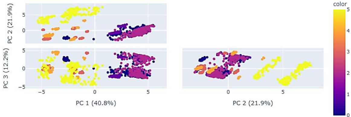
Figure 25: PCA on THz focused bins of black plastics (0:ABS, 1:PS, 2:PC, 3:PE, 4:UHMW, 5:POM)
