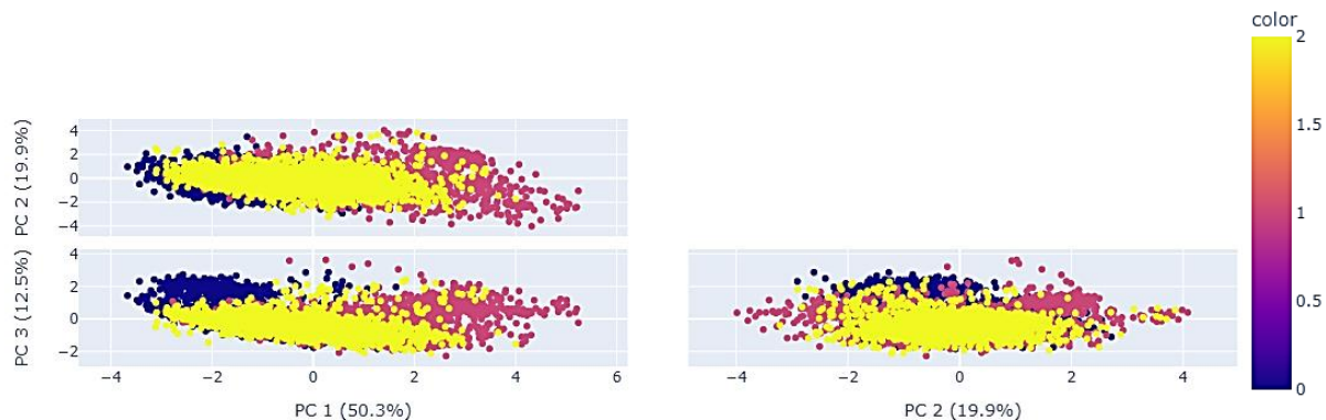
Figure 32: PCA of MWIR spectrum with focused bins (0: ABS, 1: PS, 2: PE)
