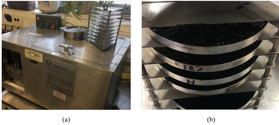
Figure 3.5: Long-Term Aging, (a) Pressure Aging Vessel and (b) Aged binders
