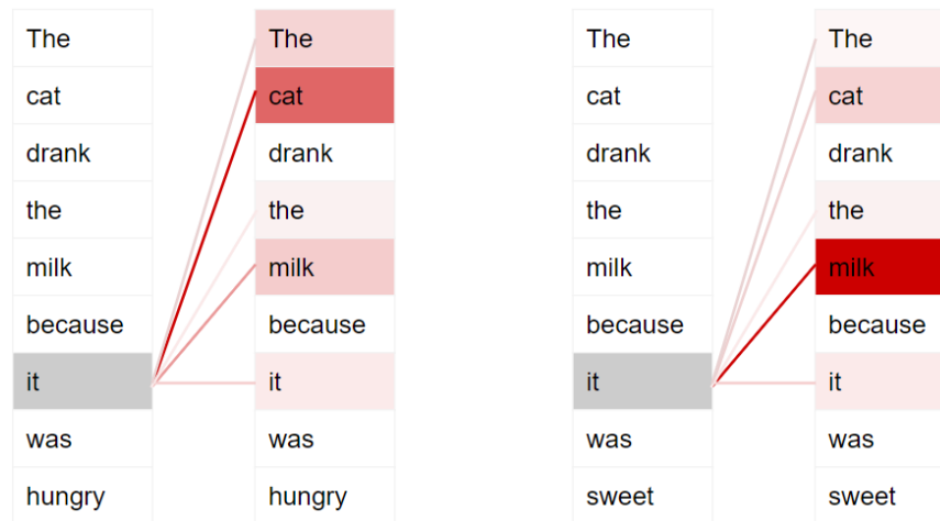
Figure 2.5 This image illustrates the self-attention weights of a transformer model. Attention weights are reflected by color intensity. The image is taken from Doshi [5]
