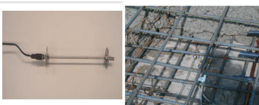
Figure 2-16 Optical fiber sensor configurations and functioning (Ansari, 2007)
