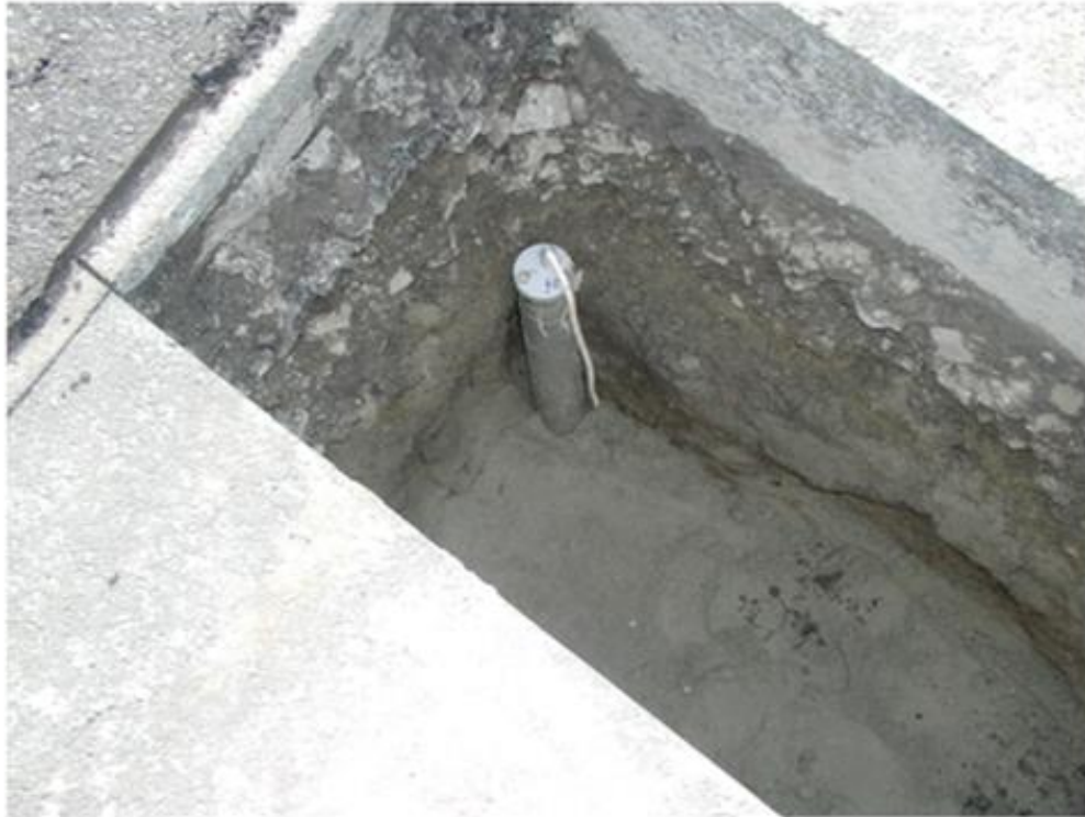
Figure 2-8 In-situ CRREL resistivity probe (Maadani, 2015)
