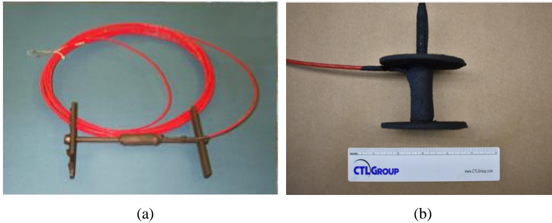
Figure 2-1 Horizontal (a) and Vertical (b) Asphalt Strain Gauges (Courtesy of CTLGroup)
