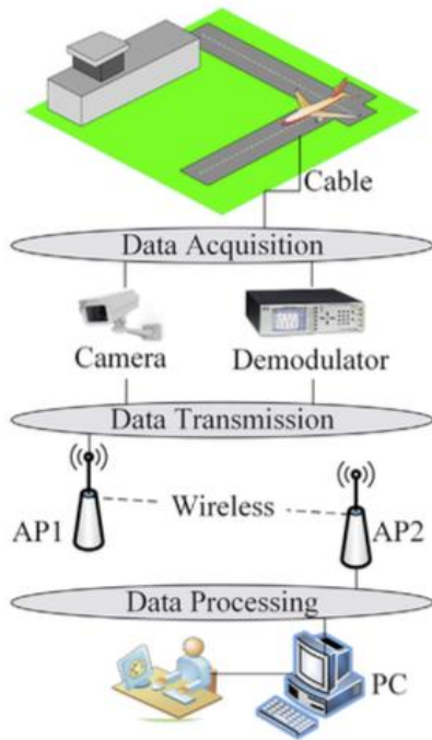
Figure 2-11 Example data acquisition system layout (Dong et al., 2017)
