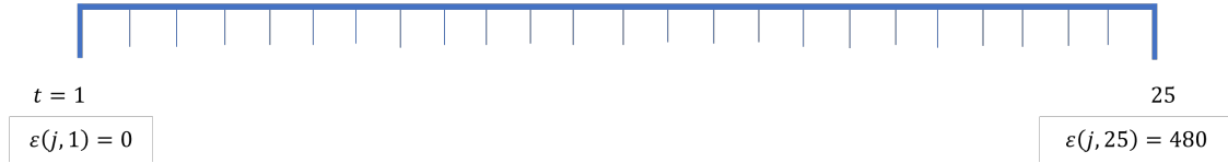
Figure 3.1: Example time discretization of a task j with \Delta(j) = 20 and a scheduling horizon of 480
