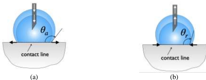
Figure 4.8: Schematic depiction of the procedure employed for the determination of (a) A.C.A. and (b) R.C.A.
