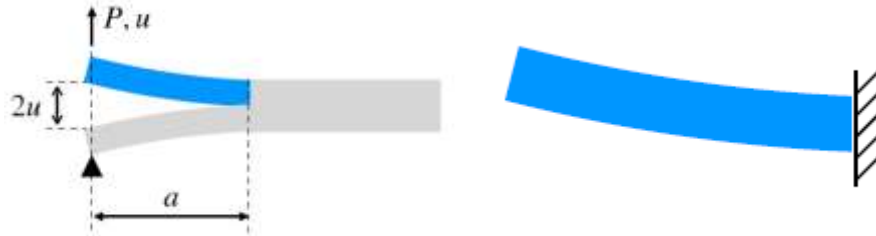
Figure 3.19: Determination of the compliance of a cantilever beam.
