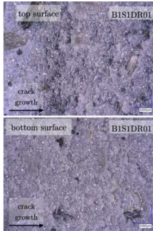
Figure 4.25: Microscopy images for ENF specimens at 0.1 mm/s (crack growth from left to right).
