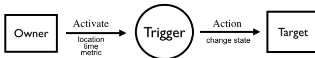
Figure 3.4: GeoScenario Trigger. When the owner activates a trigger, an action is executed on the target. The trigger can be activated when the owner reaches the trigger node location, when the Scenario reaches a certain time t , or when a metric between two agents reaches a certain value x .
