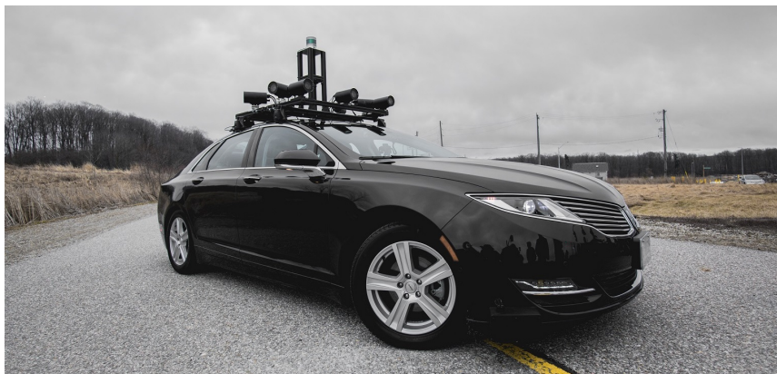
Figure 3.6: “UW Moose” research platform. Lincoln MKZ Hybrid modified to autonomous drive-by-wire operation and a suite of lidar, cameras, inertial and vision sensors.
