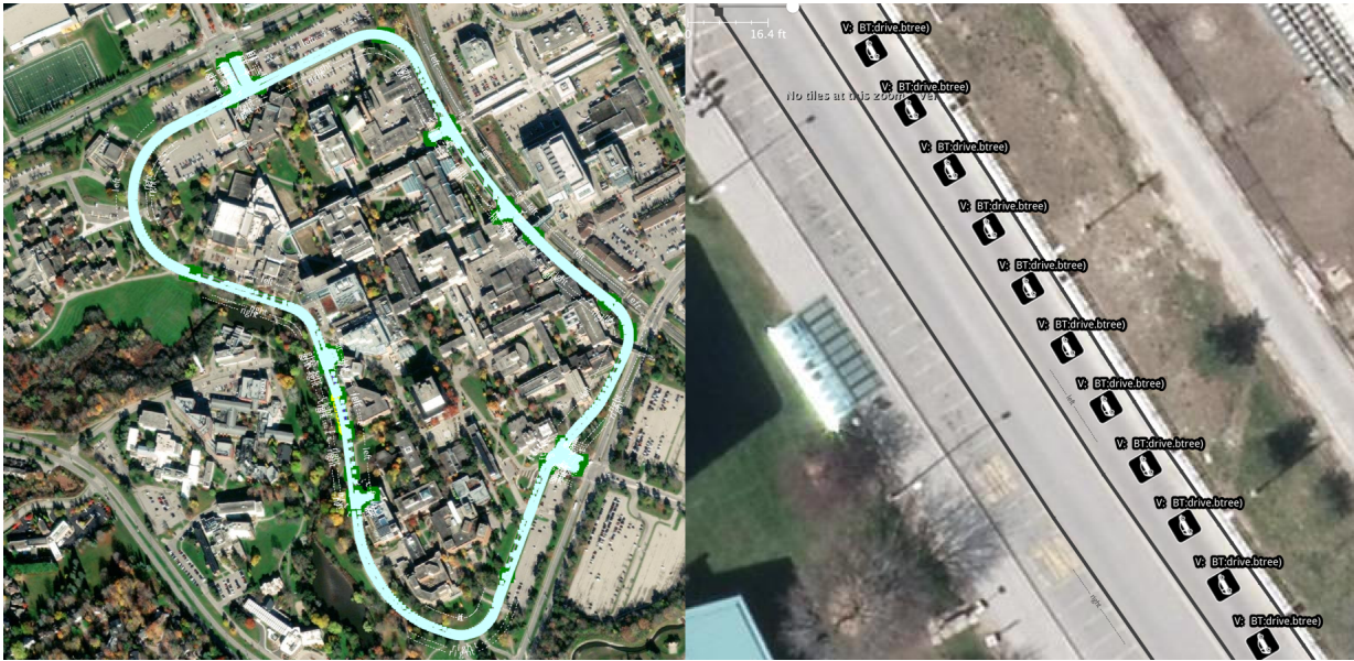
Figure 6.9: Scenario setup in GeoScenario. Up to 20 vehicles are travelling in one lane on the University of Waterloo Ring Road (lanelet map on the left). On the right the image is zoomed-in over the starting lane. The starting distance between vehicles is defined as 5m in Frénet frame.
