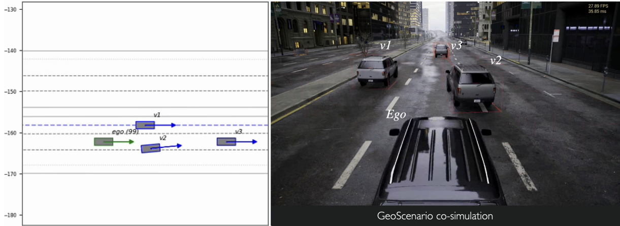
Figure 4.1: A challenging interaction between Ego and HVs based on a pre-crash scenario from NHTSA [54] and using the SDV model in simulation: (left) the SDV Model as V_2 performs the cut-in maneuver targeting Ego, and (right) a high-fidelity co-simulator renders the scene.
