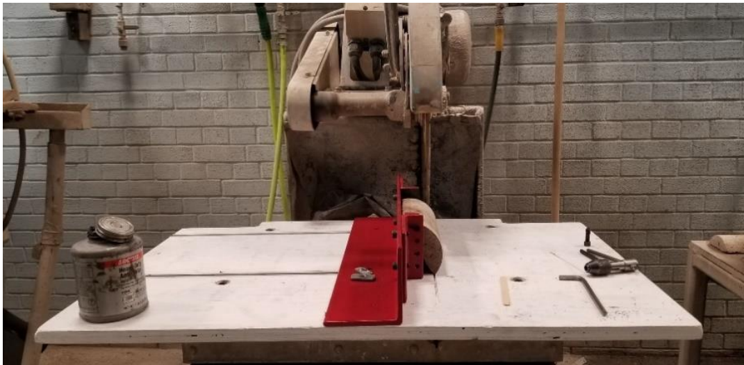
Figure 3.17 Clamping system for concrete saw table
