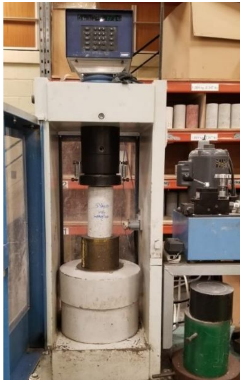
Figure 3.14 Cylinder compression strength test setup
