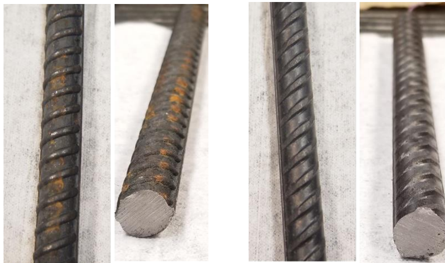
Figure 3.1 Longitudinal and sectional photographs at time of testing. (Left) Ha rebar after more than 3 years in the laboratory; (Right) MA rebar few months after dispatch from rolling mill
