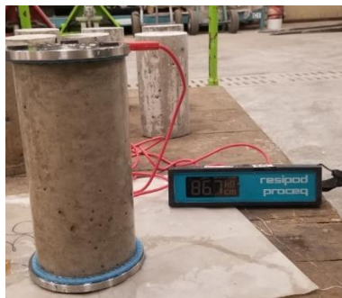
Figure 3.13 Test setup for measuring bulk resistivity of a concrete cylinder
