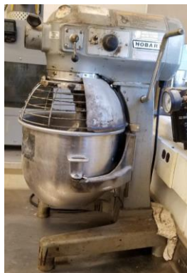
Figure 33.2 (Left) Hobart mixer used to blend the cement paste mixes; (Right) Hotdog rolling machine used for continuous rolling of cement paste cylinders
