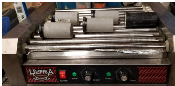
Figure 33.2 (Left) Hobart mixer used to blend the cement paste mixes; (Right) Hotdog rolling machine used for continuous rolling of cement paste cylinders
