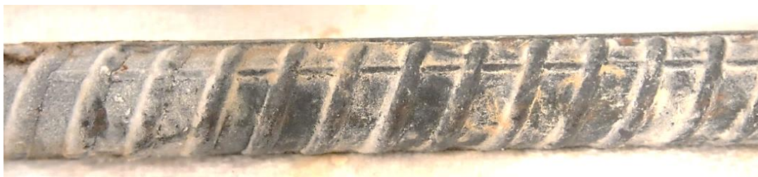
Figure 4.15 Adsorbed white precipitate coating a specimen from 0BFSGUL test solution
