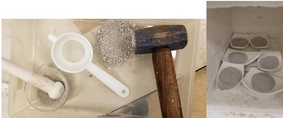
Figure 3.7 (Left) Tools used for powdering the cement paste cylinders; (Right) Ground samples, three for each cement paste cylinder specimen, in oven
