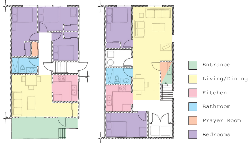
Fig. 2.15. Left to right: Room types in the Huddleston house, with a repeated entrance, kitchen, living/dining room, bathroom, bedrooms, and self-fashioned prayer room across the ground and basement floor.
