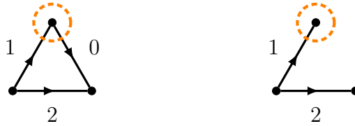
Figure 1.5: Deleting a weight 0 arc may introduce new dicuts. The right weighted digraph is produced by deleting the weight 0 arc of the left weighted digraph (arcs are labeled by their weights). The cut indicated by the dashed orange circle is not a dicut in the left weighted digraph, but is a dicut in the right weighted digraph. Furthermore, the value of \tau of the right weighted digraph is less than the value of \tau of the left weighted digraph.
