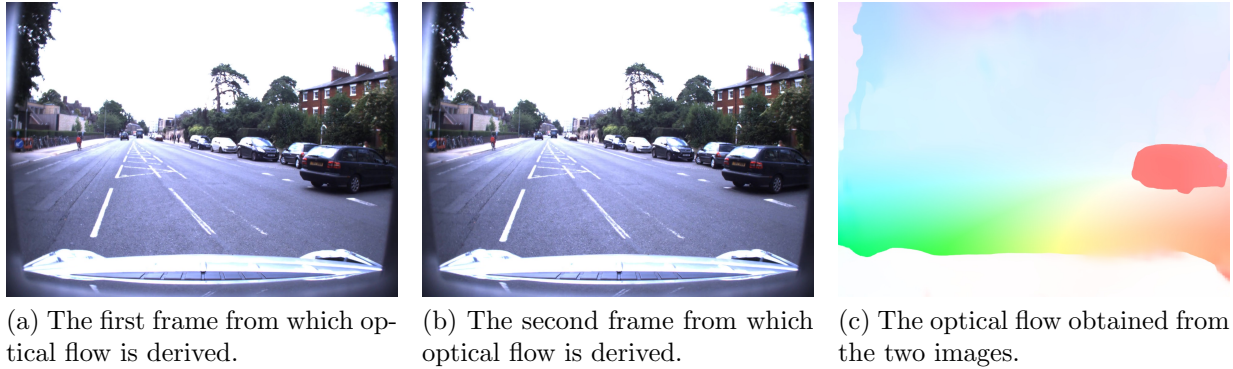
Figure 4.12: A visualization of the inputs and outputs of the RAFT network. In the output (c) the active agent can be clearly identified, unlike in the inputs (a) and (b).
