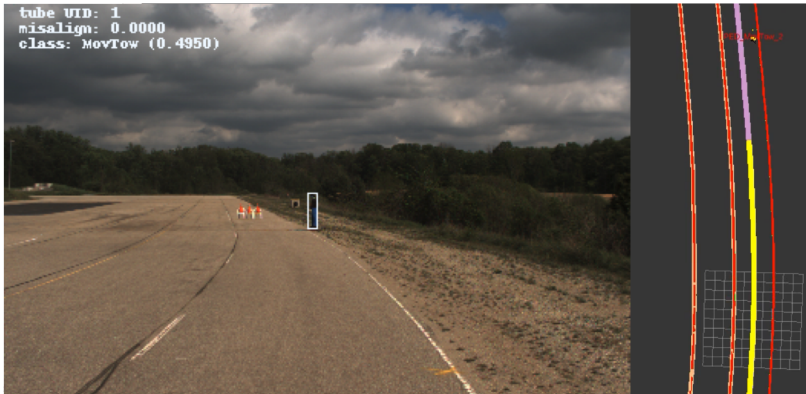
(a) Shows the overly conservative behavioral decision for the ego vehicle to stop when there is no visual indication that the pedestrian will interfere with the ego vehicle. This flawed behavior can occur when only using the geometric heuristics specified in Alg. 2, or when using an inaccurate action classifier as discussed in Section 4.3.1.
