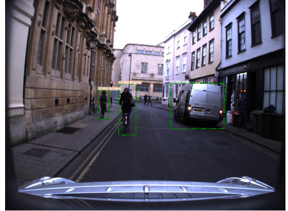
(b) A second scene where the safety of the ego vehicle is dependent on whether the idling van is stopped, or indicating that it will be entering the ego’s lane. In this case RAD-NetV1 correctly classifies the van as “Stopped”, and the ego proceeds.
