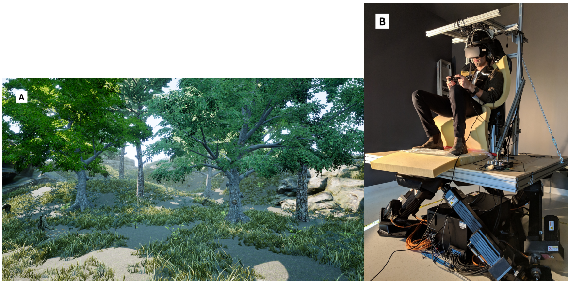
Figure 2.1: a Screenshot of the naturalistic virtual forest environment used for the visual scene in the experiment. b Physical setup of the experiment with the 6DOF motion platform, the racing seat with added foam, helmet and Oculus Rift CV1 HMD.
