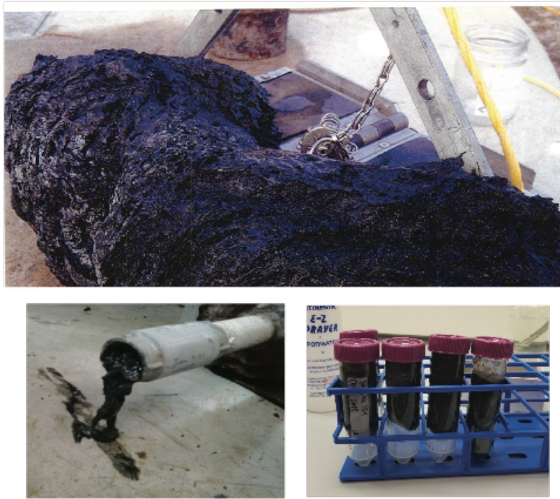
Figure 2.1 Examples of biofouling occurring at the municipal waste management site.
