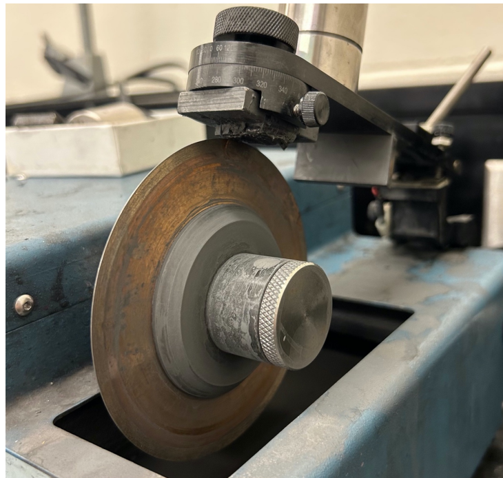
Figure 7. Diamond coated copper cutting disc setup. Samples are hot glued to the plate.
