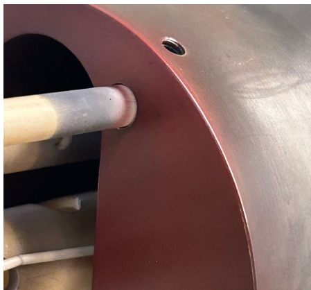
Figure 61. Se condensation in the ZEM instrument, characteristic result of measuring unstable samples with excess Se.
