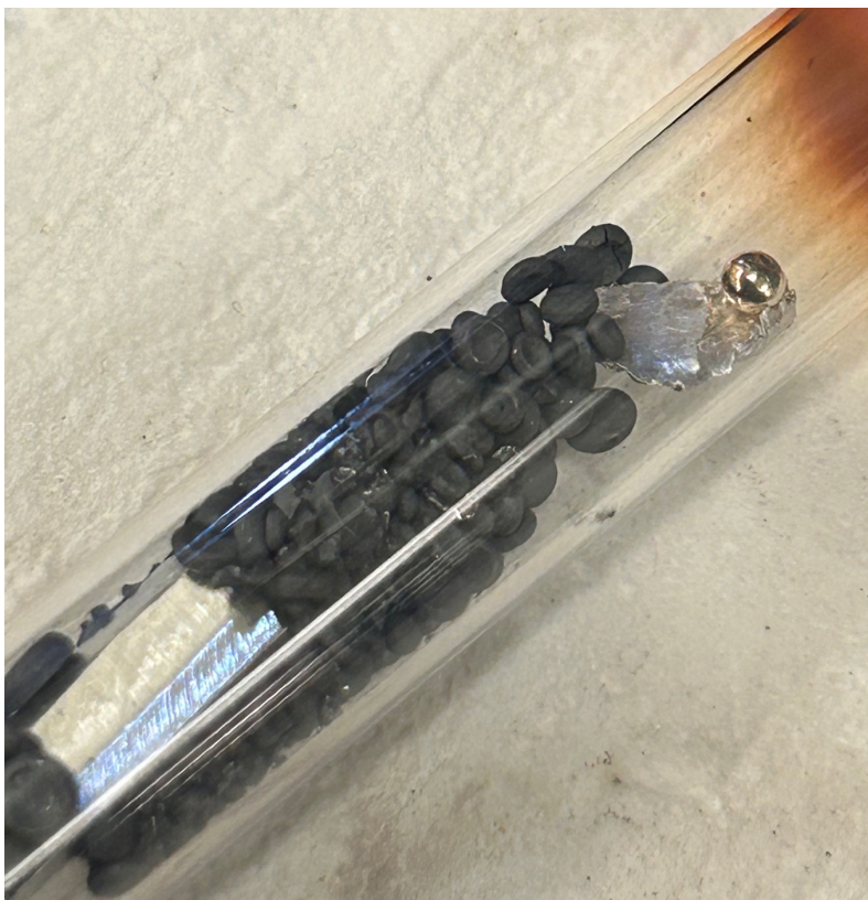
Figure 86. The weighed out and double vacuum sealed Na, Sn, Ag, and Se for the samples with the composition \text{Na}_{0.033}\text{Ag}_{0.016}\text{Sn}_{0.963}\text{Se} .
