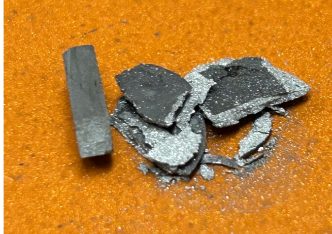
Figure 80. Grain growth visible from TD measurement (left is before, right pieces are after TD).
