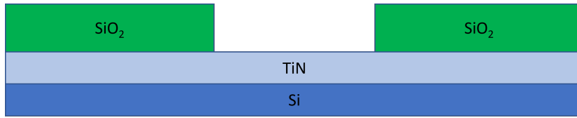
Figure 4.6: Sketch of the side view of device area(white square zone in Figure.4.7). The TiN is the bottom electrode and the device size is defined by SiO_2 .
