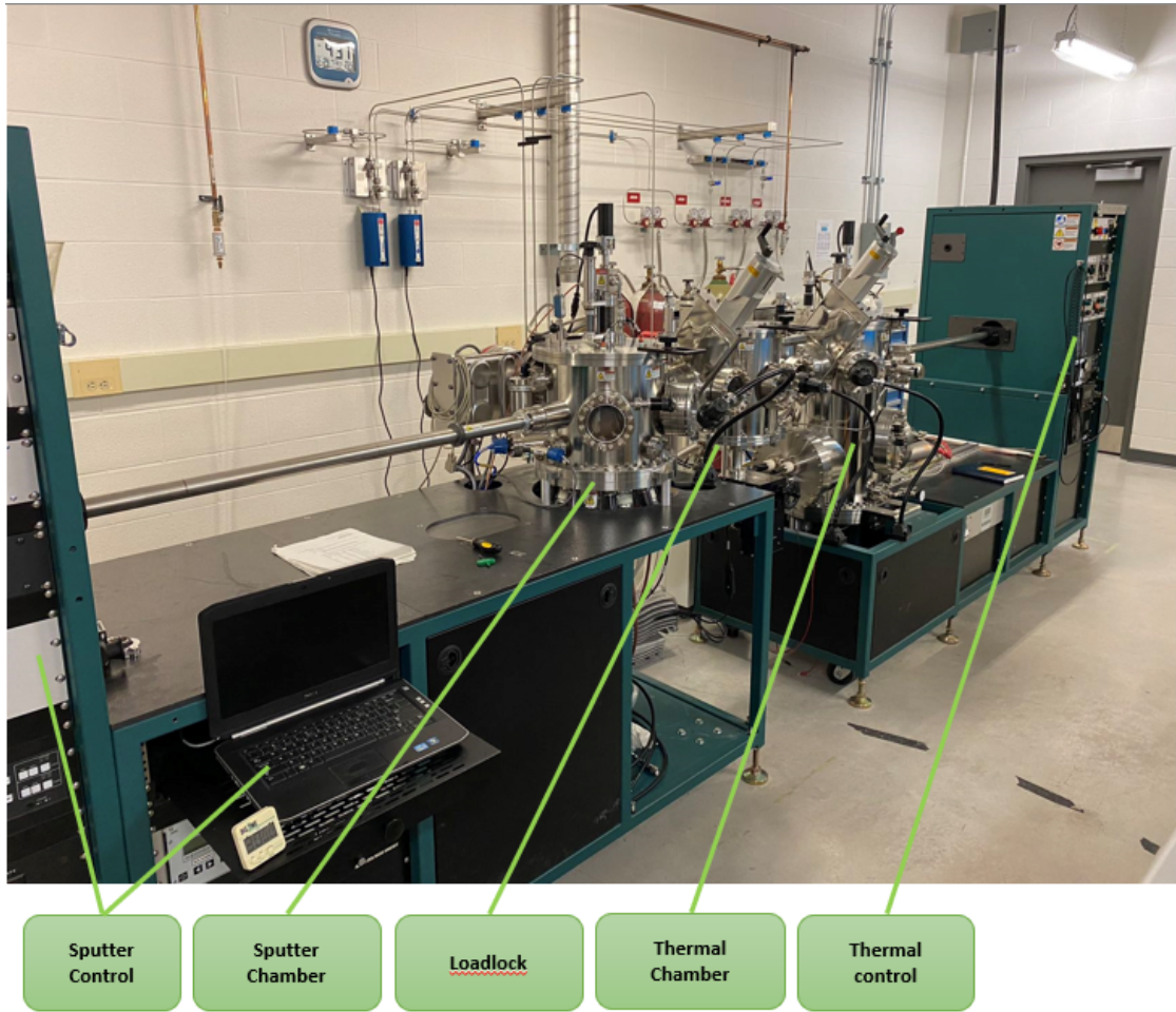
Figure 4.10: AJA Twin Chamber system overview
