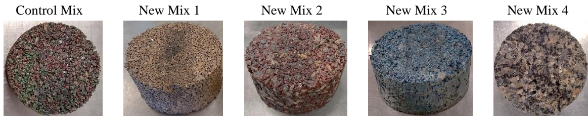
Figure 53 Permanent deformation due to rutting on different mixes
