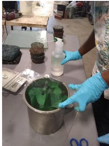
(b) Vacuumed-sealed sample placed into the container
