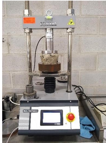
Figure 40 Test equipment for Unconfined Compressive Strength (UCS)
