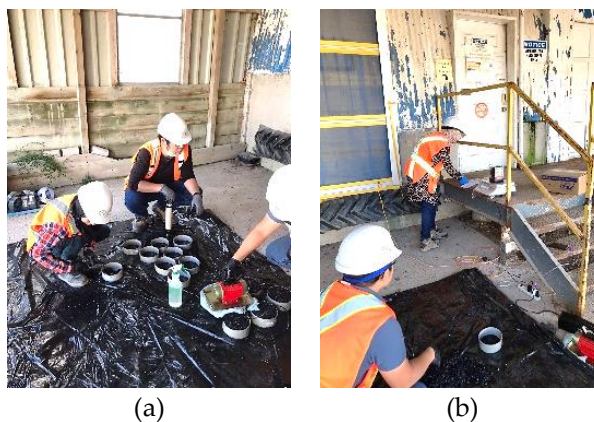
Figure 76 Preparing sample from trial section mixes; (a) Pouring material into the molds, (b) Weighing the material for pouring into the mold
