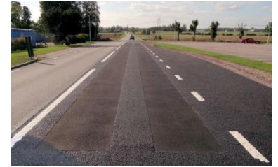
(c) Test tracks in Linköping, Sweden, were laid in August-September 2014, with prefabricated panels (front, 30 m) and on-site construction (rear, 24 m)
