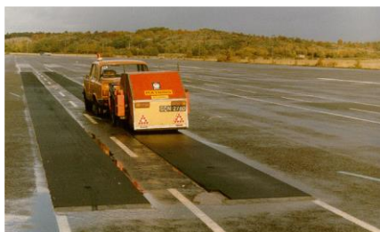
(b) Strips of PERS laid on closed down Torslanda Airport in 1984
