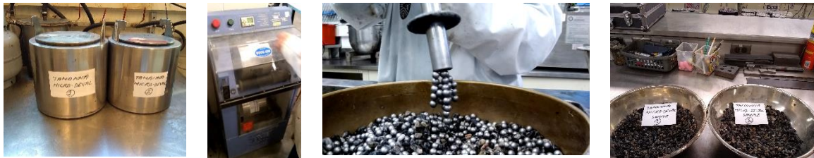
Figure 52 Micro-Deval abrasion loss test at the lab
