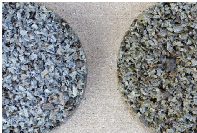
Figure 14 Ambering in PRP after curing
