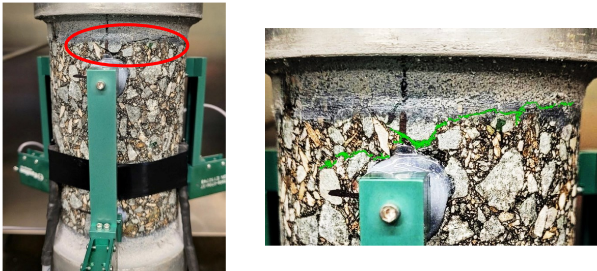
Figure 10-20 Left: Specimen with visible macrocrack on the surface of a Gr2x-125 replicate (using an initial strain of 125 µm/m with an 8-hour rest period). Right: Close-up image with the macrocrack highlighted in green.
