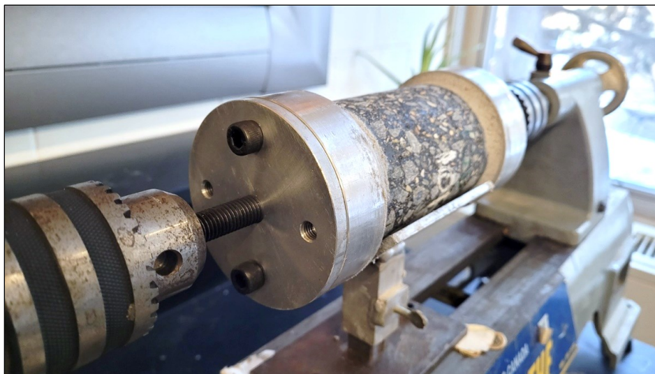
Figure 8-2 End-plate gluing jig constructed from a repurposed wood-turning lathe.
