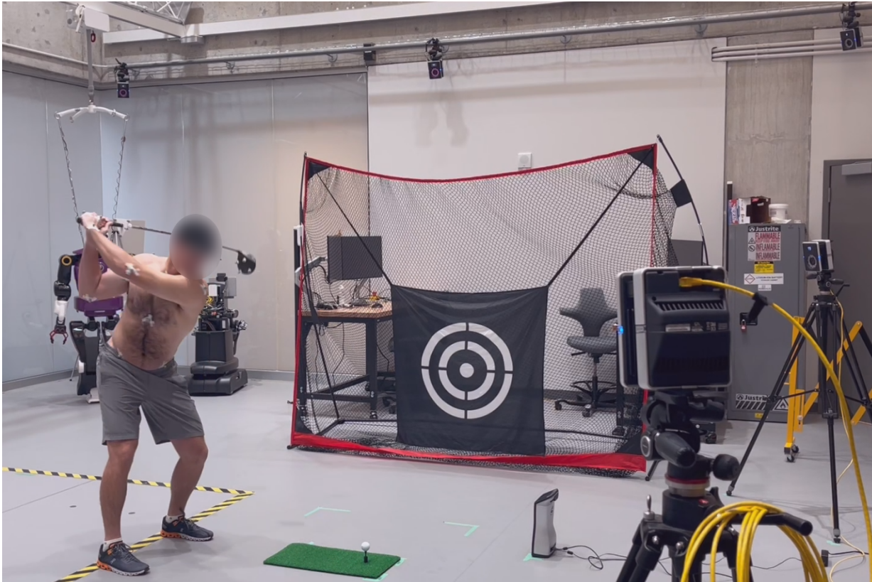
Figure 4.1: Motion capture study participant Golfer 5 at the top of backswing position. Markers can be seen affixed to the participant's pelvis, torso, and upper extremities as well as on the grip and head of the golf club. A Foresight Sports GCQuad launch monitor is present to the right of the golf ball to record launch conditions. Five of the 13 VICON Vantage cameras used are visible along the upper wall and mounted on tripods.
