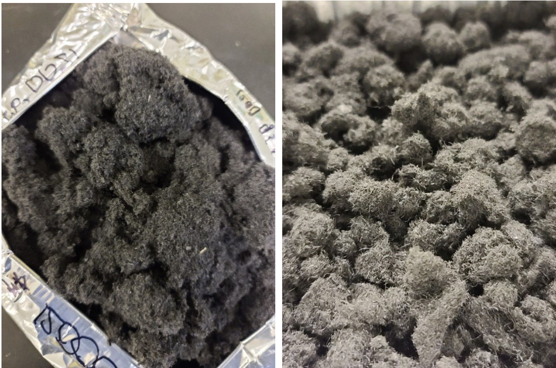
Figure 3-3 Milled sample "cake" [left] vs pelletized form [right]
