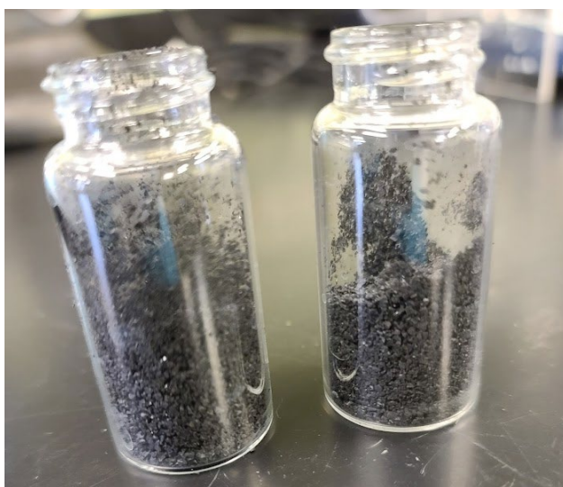
Figure 3-5 Fine pellet sample obtained after high RPM grinding of the extrudate, prior to MFR testing.
