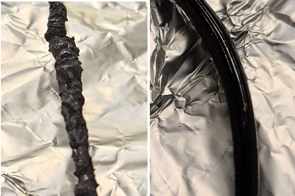
Figure 4-2 Comparison of the same extrudate strand with heterogeneous mixing. The strand on the left demonstrates the sharkskin defect and the strand on the right is perfect.
