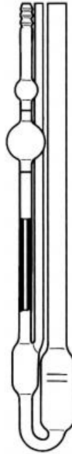
Figure 2-16 Schematic of a standard Ubbelohde viscometer. (SI Analytics TM Ubbelohde Viscometers for Manual, n.d.)
