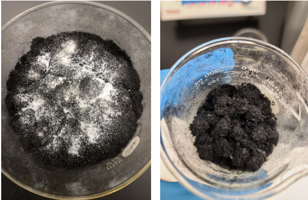
Figure 4-3 Comparison of extruder feed stock when un-pelletized [left] and pelletized [right]
