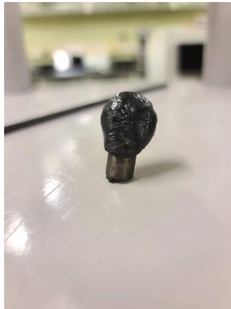
Figure 4-4 Die blockage due to testing temperature being too low at low/low formulation ( T_{MFR} = 250^{\circ}\text{C} )
