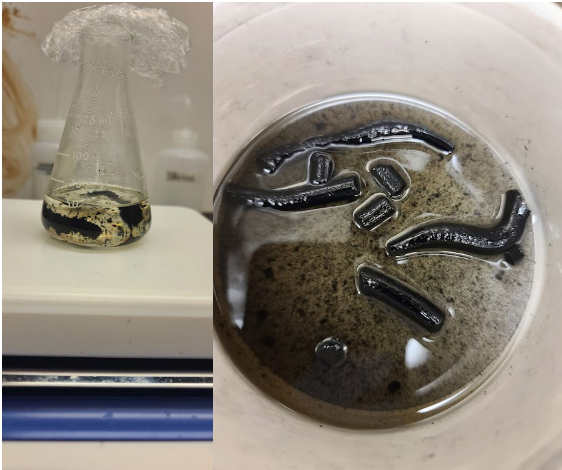
Figure 4-6 Carpet trim inside the 60/40 solvent [left] and carpet trim swelling due to gel formation [right]
