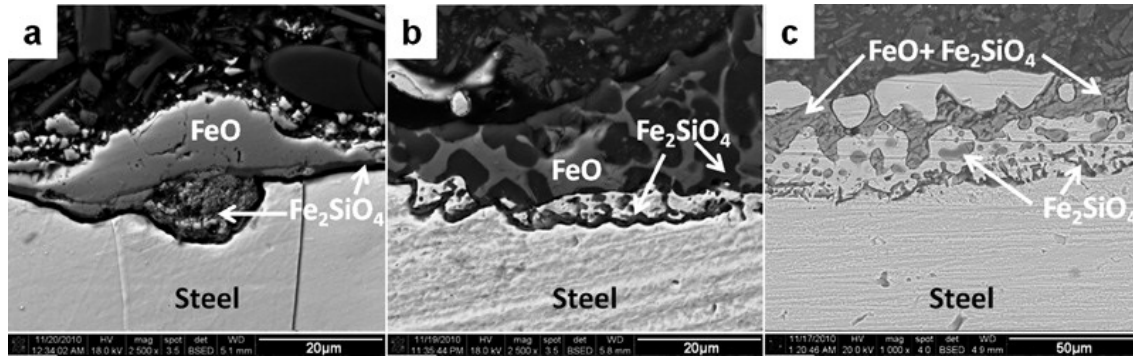
Figure 12: SEM images of silicon steel oxidized for 20 minutes at (a) 950°C (b) 1100 °C (c) 1150°C [20]
