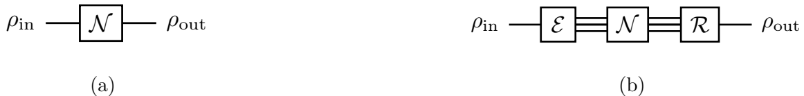
Figure 6.2: (a) Quantum communication model where Alice sends a state \rho_{\text{in}} to Bob through a noisy channel \mathcal{N} . (b) An attempt to reduce the effect of \mathcal{N} using QEC, through an encoding operation \mathcal{E} and a recovery operation \mathcal{R} .
