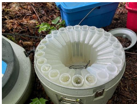
Successful ISCO collection of a set of event-scale stream samples
