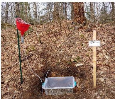
Throughfall collector in C32, March 2021
