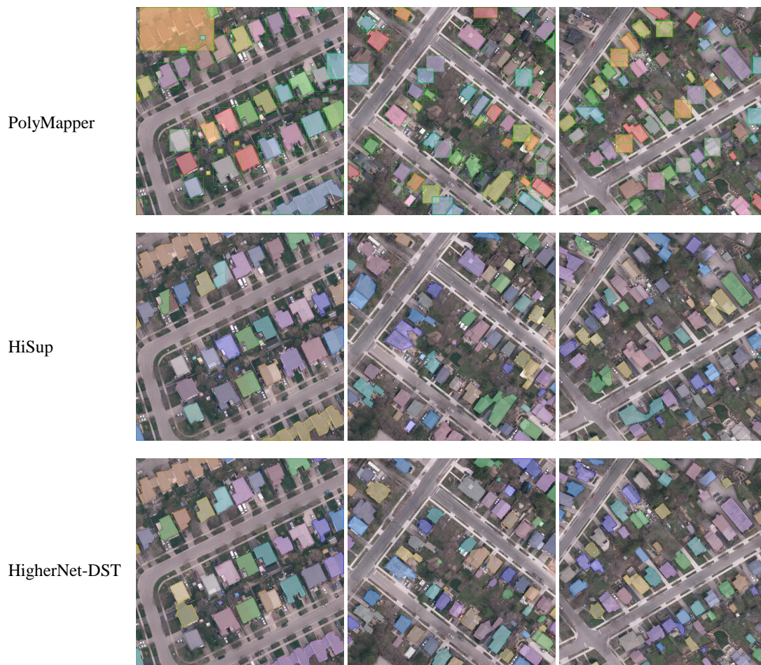
Figure 4.8: Rooftop delineation results on the Waterloo Building Dataset (top: results from HiSup, bottom: results from HigherNet-DST)
