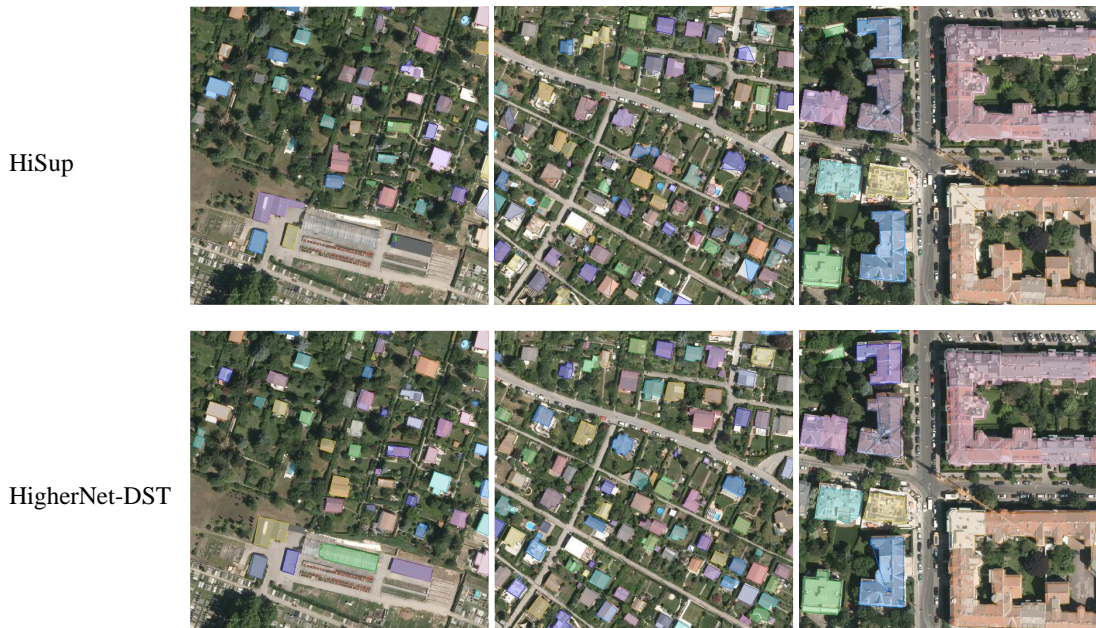
Figure 4.5: Building polygon delineation results on the Inria Building Dataset (top: results from HiSup, bottom: results from HigherNet-DST)
