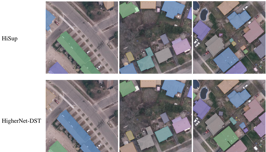
Figure 4.7: Rooftop delineation results on the Waterloo Building Dataset (top: results from HiSup, bottom: results from HigherNet-DST)
