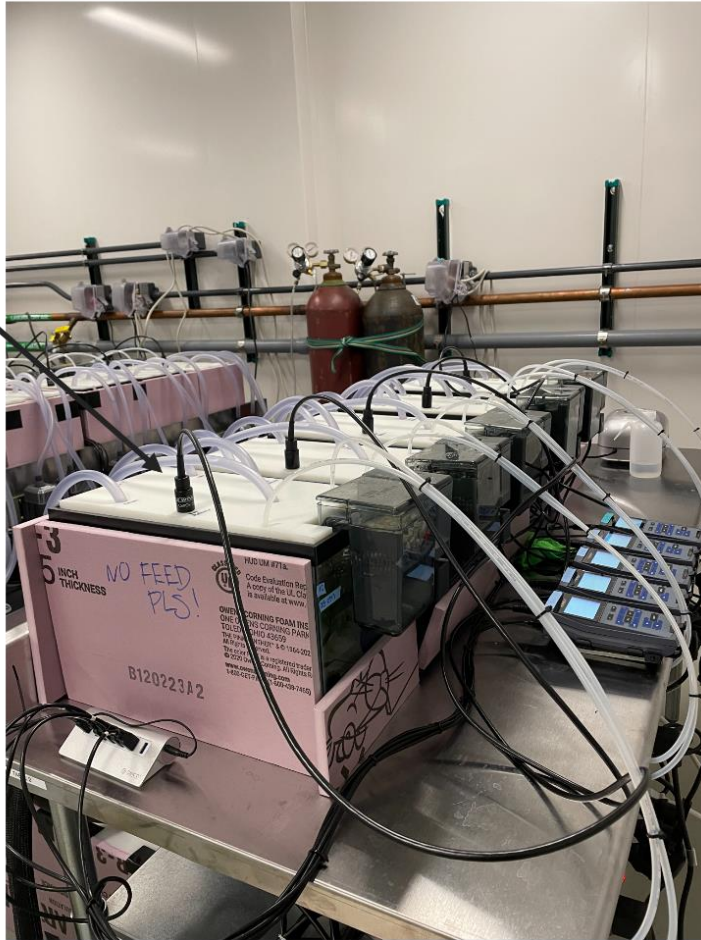
Figure 0.3 In-lab tank set-up for 15 d acclimation exposure.
