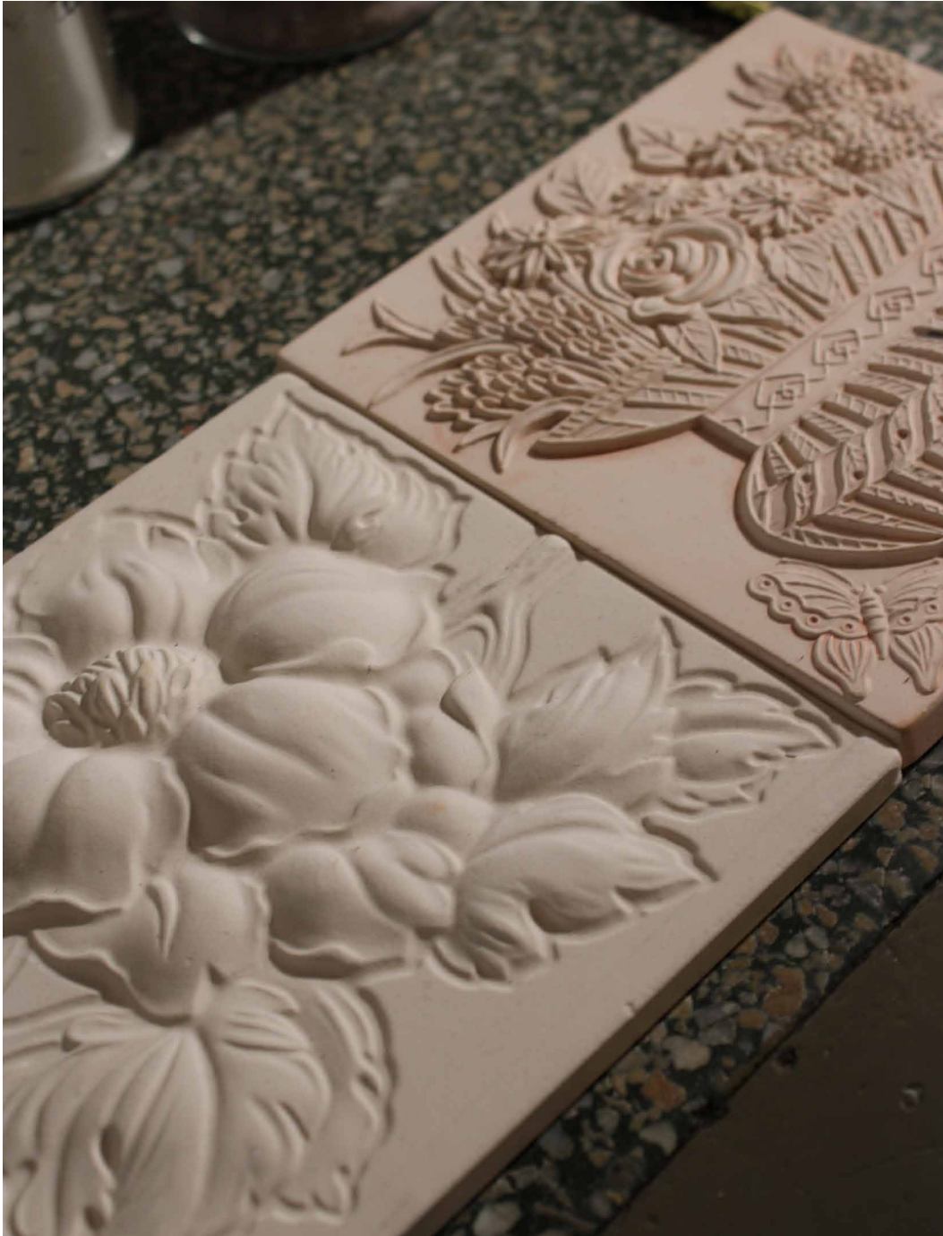
Fig. 6.94 The molds for each Majolica tile pattern is hand carved by the artisan before they are used for printing.
