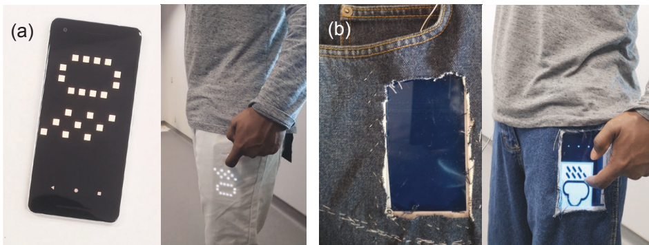
Figure 3.8: User study baseline device conditions: (a) a standard phone with high contrast pixelated imagery; (b) a futuristic PDLC transparent pocket to make a standard phone display completely visible “through fabric”.
