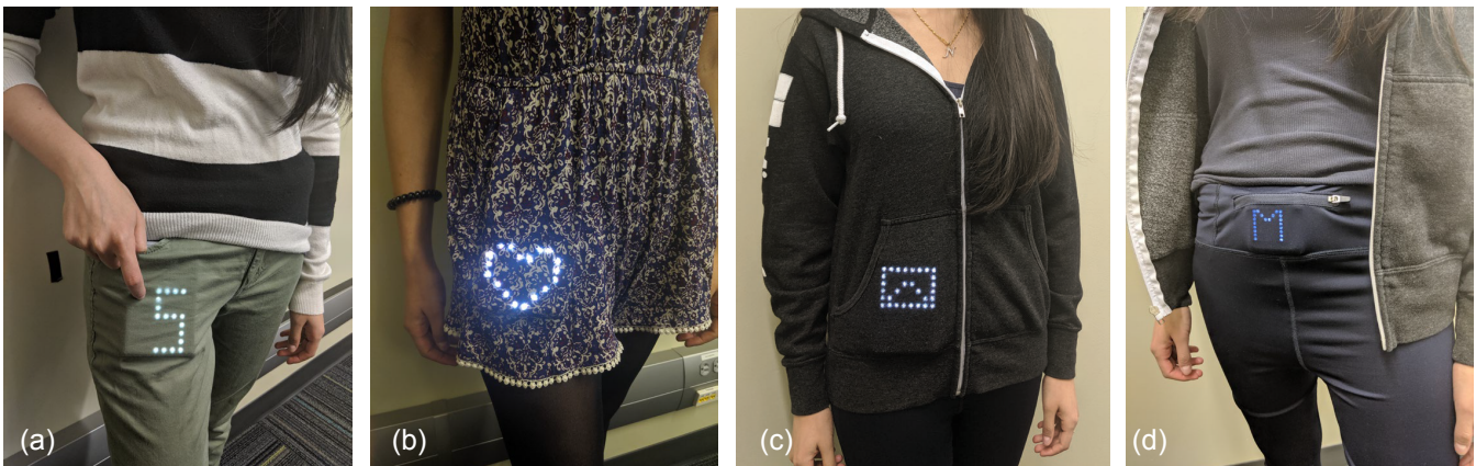
Figure 3.7: Interaction vocabulary imagery demonstrated with different kinds of clothing and pockets: (a) numeral 5 through cotton pants; (b) fitness icon through knit dress; (c) mail notification icon through hoodie; (d) message notification icon through front pocket of lycra tights.
