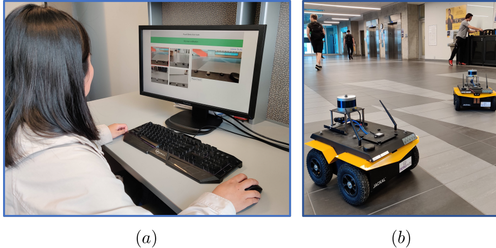
Figure 6.1: Multi-robot supervision user study setup: a) A participant monitoring multiple robots using the web-based interface, b) Clearpath Jackal robots used for the study.
