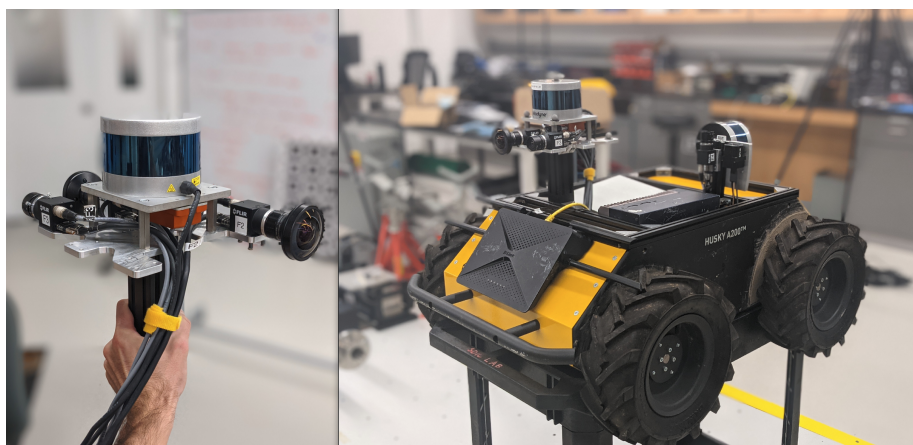
Figure 1.1: Infrastructure scanning data collection platforms. (Photos by: Nicholas Charon)
