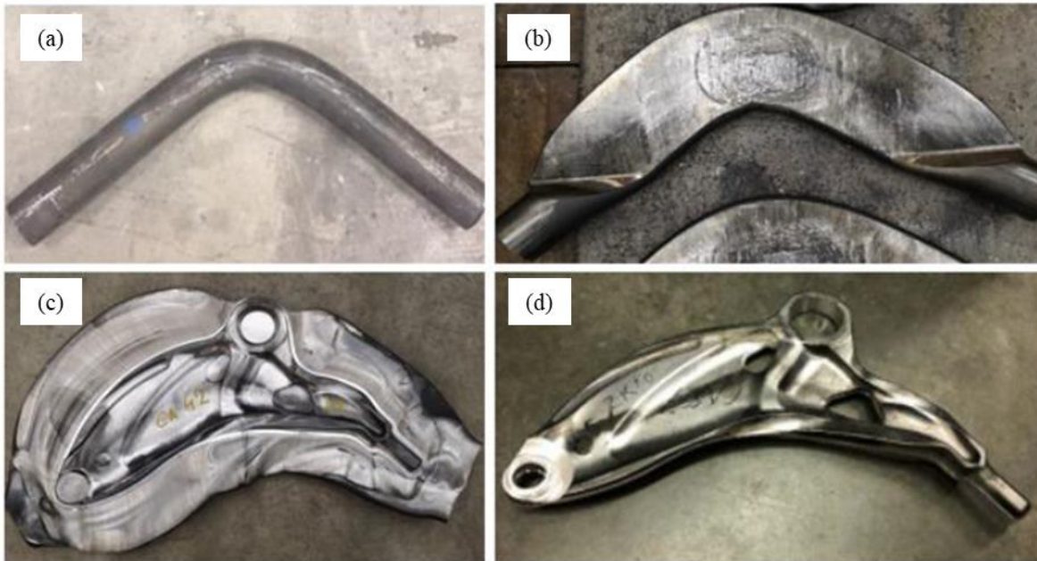
Figure A-2: The AZ80 alloy front lower control arm that was forged during the APC project; the multiple pre-forming steps are shown in: (a) bent Mg alloy billet; (b) flattened preform shape; (c) as-forged FLCA; (d) FLCA with flash trimmed and surfaces machined.
