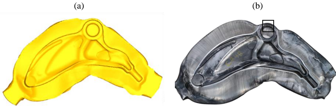
Figure 3-12: (a) Control arm forging simulation; (b) laboratory-scale forging of CA48 with a 2 mm underfill at the bushing in the indicated region.
