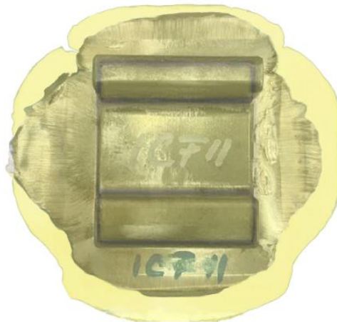
Figure 3-10: I-beam simulation and laboratory-scale forging flash comparisons.
