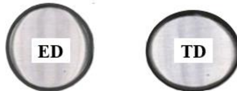
Figure 2-5: Wrought samples compressed along the ED and TD directions (as viewed from the compression direction) at 400°C at a strain rate of 0.1 s -1 to a strain of 1.0 (wrought AZ80 alloy).
