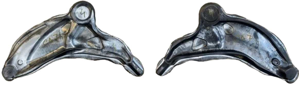
Figure C-6: Control arm forging outcome using cast-preform iteration 11 (CP11), forged under 300 °C temperature condition (courtesy of CanmetMATERIALS, Bruce Williams)
