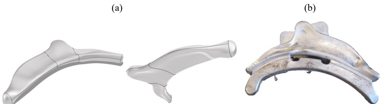
Figure C-3: (a) Control arm cast-preform design iteration 11 (CP11); (b) cast preform (courtesy of CanmetMATERIALS, Lucian Blaga).
