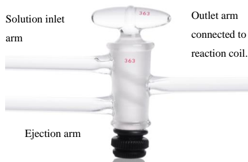
Figure 2.3: Photo of a three-way valve with oblique bores, and three arms.
