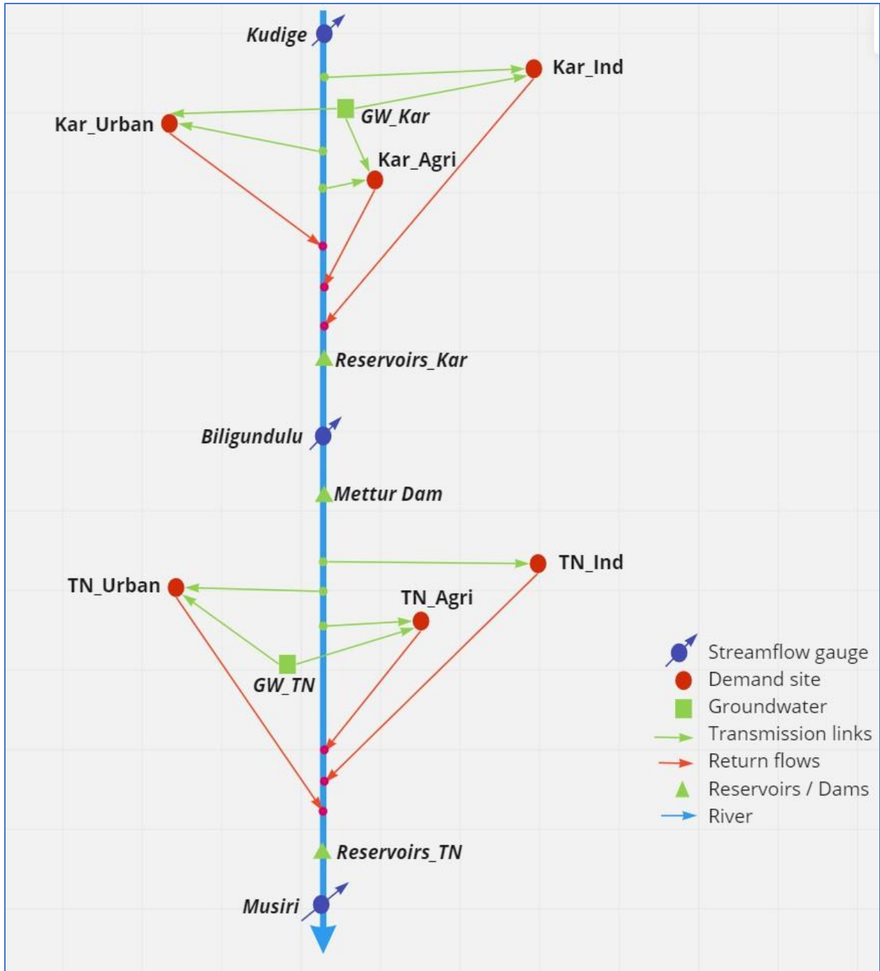
Figure 23 Simplified schematic of the Cauvery River basin model with WEAP elements.
