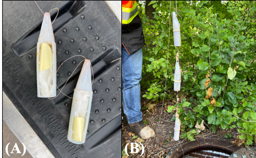
Figure A-2. Triple torpedo sampling apparatus (A) loaded with electronegative membrane filter and medical gauze, and (B) sampling apparatus immediately following collection.
