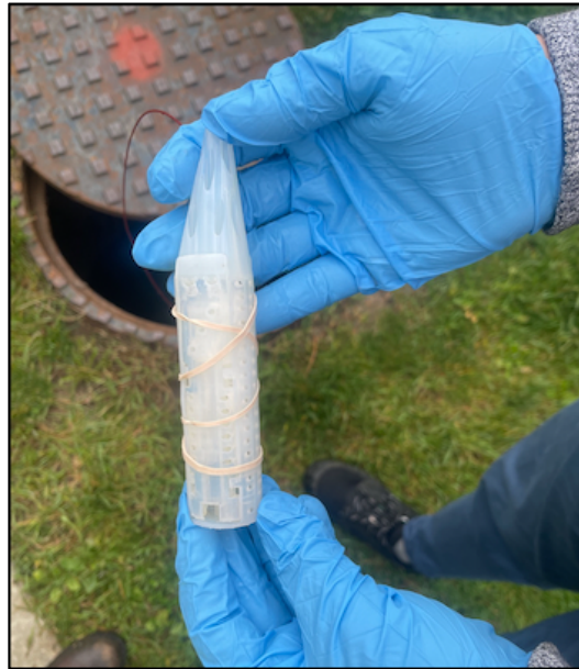
Figure A-6. Passive sampling apparatus prior to deployment: A torpedo-shaped housing vessel (Schang et al., 2021) loaded with cotton gauze and secured by an elastic band.
