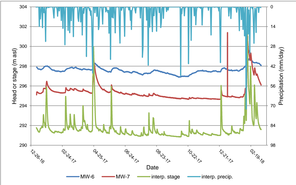
Fig. 9 HLDTc hydrographs for MW-6 and MW-7, with interpolated river stage, January 2017 to March 2018 (Sherman, 2019); average daily precipitation was averaged from USGS gage stations Pineville (03402900) and Barbourville (03403500)
