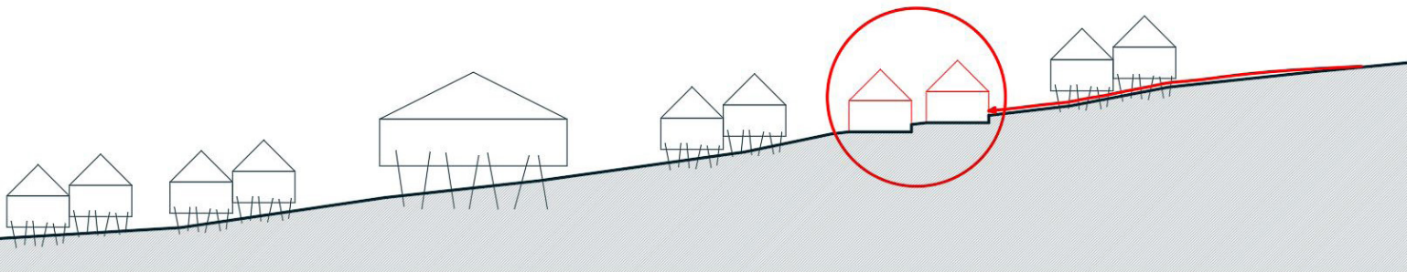
Figure. 3.15. Using traditional stilted building techniques is essential to avoid triggering lethal mudslides, flooding, and other natural disasters when constructing terraces. Bottom right diagram illustrated by Author.
