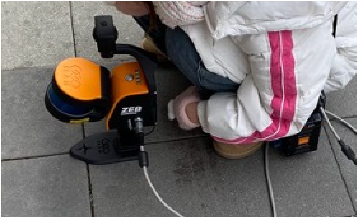
Figure 5.15: GeoSLAM laser scanner operation during data collection
