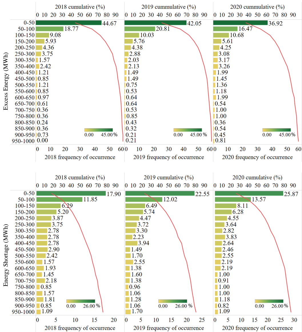
Figure 3.4: Annual frequency distribution of capacity requirement for excess power (upper), and power shortage (lower) in Ontario for three years of 2018, 2019, and 2020. The red lines depict the cumulative frequency of occurrence (%).
